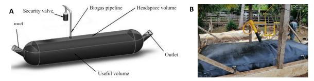
Figure 7: Schematic of a basic design of a tubular-type digester, taken from Garfi et al. (2016) (**A**). An image of a working tubular digester from <a href="https://www.permaculturenews.org/2020/10/23/biogas-and-carbon-farming-part-3/ml">https://www.permaculturenews.org/2020/10/23/biogas-and-carbon-farming-part-3/ml</a> (**B**).
