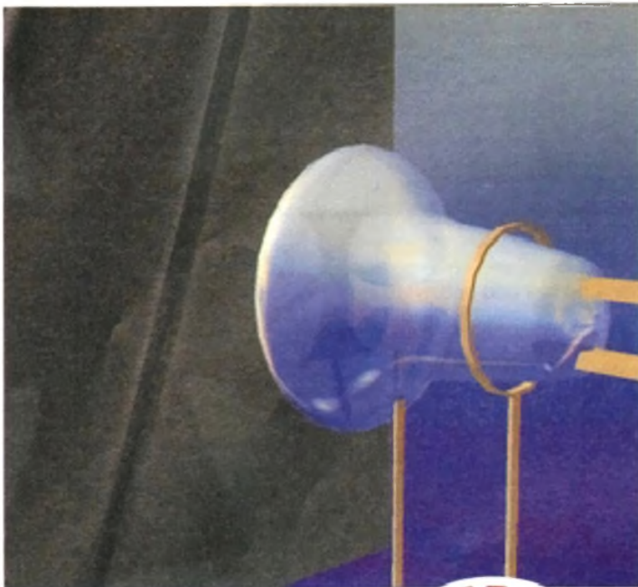
This early design of cathode ray tube shows a Maltese cross working as the anode, projecting its image onto the screen
