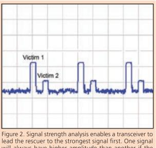
lead the rescuer to the strongest signal first. One signal will always have higher amplitude than another if the rescuer is moving.
