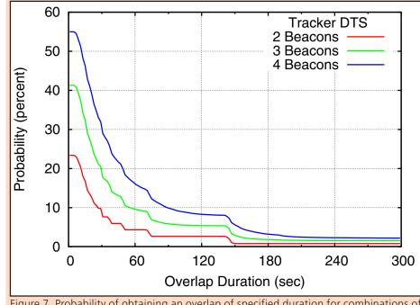
Figure 7. Probability of obtaining an overlap of specified duration for combinations of two, three, and four tracker DTS beacons.
