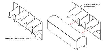
5 Complete the installation by ensuring the louver is consistently aligned across the round shape of the lens.
