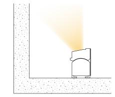
3 Before installing, place louvers on fixture in sequence to determine positioning and spacing.
