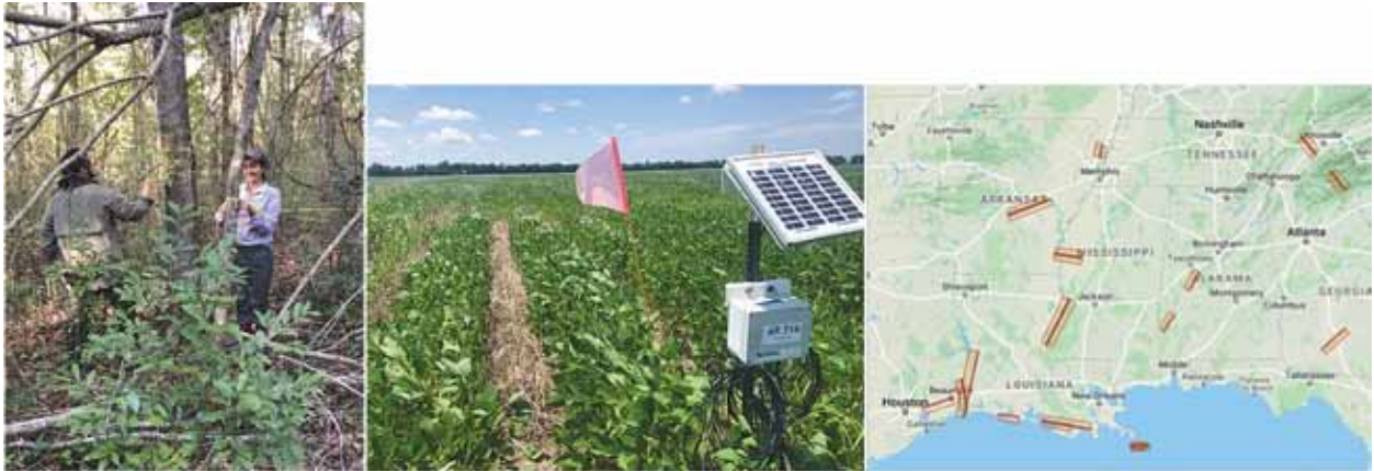
Figure 26. Left: JPL scientists Neda Kasraee and Adam Vaccaro survey a vegetation plot in Alabama during the NISAR AM/PM campaign. Photo credit: Victoria Meyer / JPL, Center: Data loggers record soil moisture measurements at a farm during the NISAR AM/PM campaign. Photo credit: Nathan Torbick / Applied Geosolutions. Right: UAVSAR coverage during the campaign flown on the JSC G-III.
