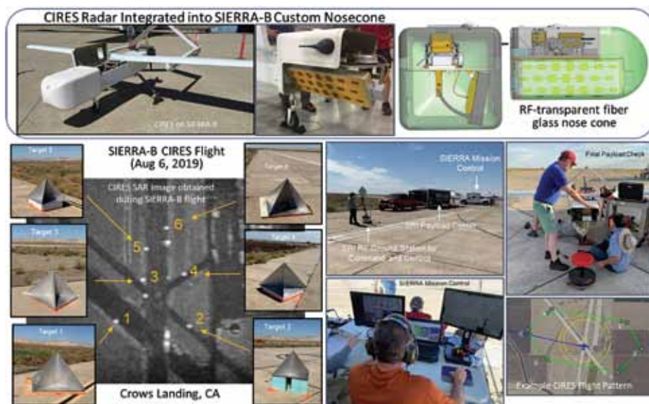
Figure 30. Top: CIRES was integrated into the ASP SIERRA-B UAS using a custom-built nose cone. Bottom: CIRES flew on SIERRA-B over Crows Landing, California in August 2019, obtaining the payload's first interferometric UAS-based verification data. The team deployed six radar calibration targets for characterization of CIRES height deformation measurement capabilities. Image credit: Lauren Wye / SRI
