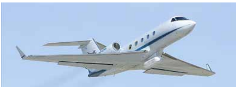
Figure 44. The JSC G-III Showing the UAVSAR Pod.
