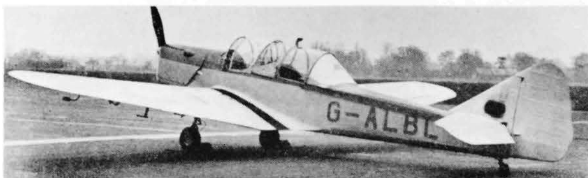
Top: The 1st production Fairey Primer G-ALBL being re-engined with Cirrus Major 3. Note the wing root spoiler strips and interim bipod crash pylons. Above: G-ALBL, now with Cirrus Major, and with spats removed. (Fairey) Left: Primer G-ALBL in its final form with the fuselage fairing behind cockpits removed. (All three via Jack Meaden)
