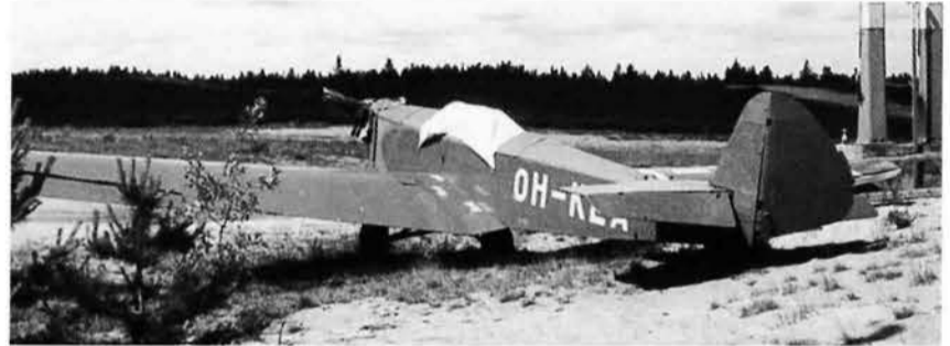
Below: Klemm L.25 OH-KLA with Poinard engine and modified rudder shape seen at Jämi in 6.54. See extract for 20.10.49. (Eino Ritaranta)
