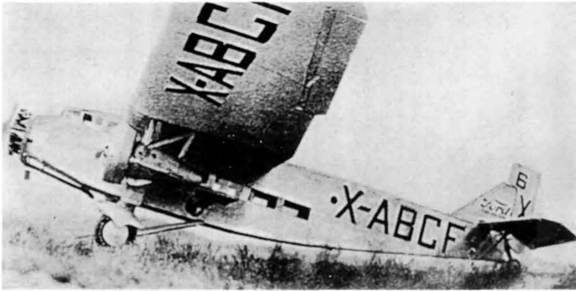
Left: Johnson Flying Service Ford Trimotor 5-AT-40 N69905 which crashed 17.8.53 was earlier used as seen here between 1.29 and 1.36 by Cia Mexicana Aviacion SA as X-ABCF. It was only purchased by Johnsons on 1.8.53 and had been converted in 1952 to 450 hp Wright R-975-28 engines in place of the P & W engines used by all other 5-ATs and seen in this view. It is speculated that the new installation may have involved changes to the fuel cock settings resulting in starvation just after take-off if the pilot was unfamiliar with the revised system. (via Jack Meaden)
