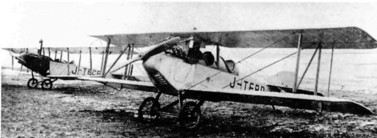
Left: The Itoh Emi 23 Bulldog trainer J-TEBD was modified from a Barr Flying Circus Standard biplane. While being flown by Takamoto Yoshikawa it stalled in a low turn and crashed into the sea. Yoshikawa was killed and passenger Taizo Tashiro badly injured. J-TECE on the left is an extensively modified Curtiss JN-4, probably also an ex-Barr machine.
