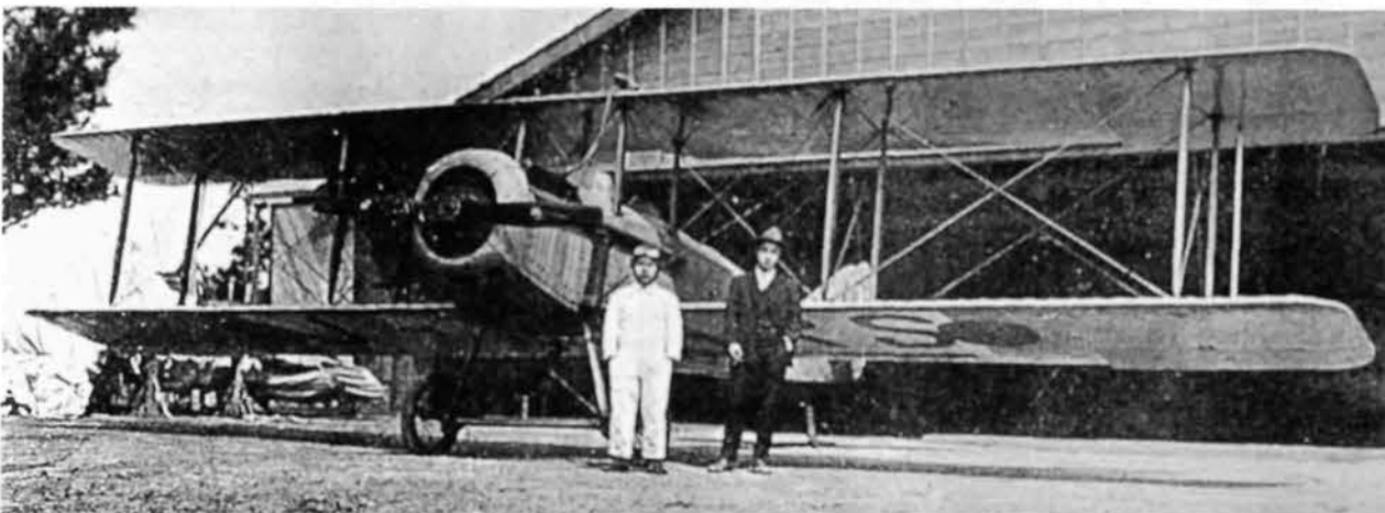
Left: The Fukunaga brothers Shiro (pilot) and Asao (designer) with their Tenryu 6 racer J-TARS with circular-cowled Hispano engine. For extended range it was converted to a single-seater with a fuel tank in the front cockpit.
