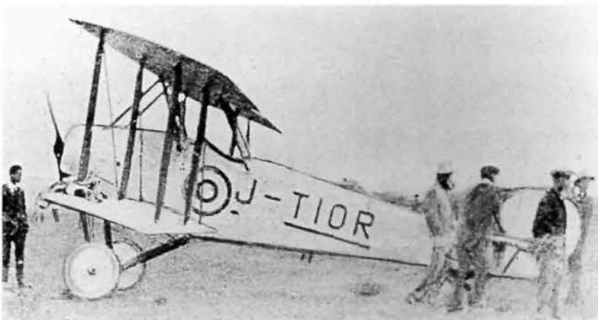
J-TIJ# Fukunaga Tenryu Type 7 2-seat open-cockpit biplane trainer (80-93 hp Le Rhone 9-cyl rotary) Designer Tomizo Asami. 11.21. One only.
