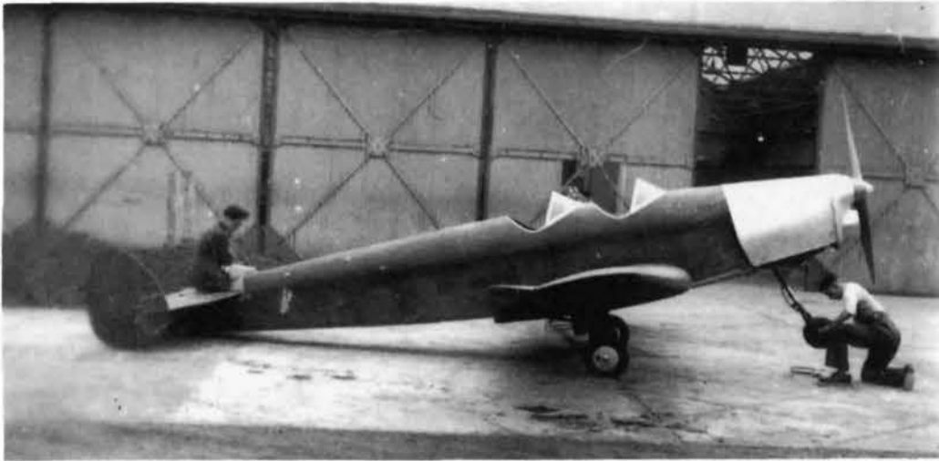
Above: The tricycle-gear Moth Minor receiving nosewheel attention while the tail is held down by the weight of designer Phil Smith.
