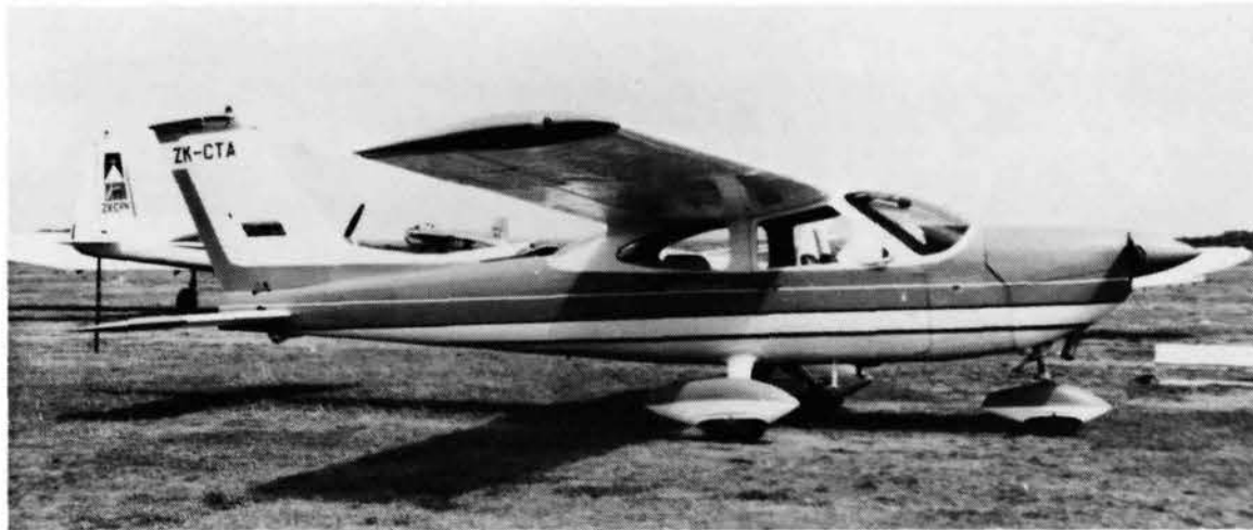
Left: The first Cessna 177 registered in New Zealand was ZK-CTA. The Model 177 was originally designated 172J and was the first of the high-wing series to feature the unstrutted cantilever wing. The de luxe version was known as the Cardinal, ZK-CTC being an example. Visible to the rear is James Aviation Fletcher FU-24 ZK-CPN. (R W Kerr)
