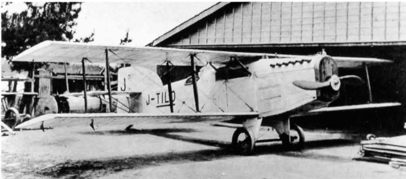
Above: J-TICE, the Nakajima B-6, was a licence-built Breguet Br 14 with a Rolls-Royce Eagle engine. Left: J-TILO, the Fukunaga Tenryu 10, was entered in a competition 6.23 with a 500 litre (110 gal) fuel tank in the cabin in place of the 4 passenger seats. Far left: J-TIOR, the Shirato 40 2-seat trainer, became a single-seater with an additional fuel tank in the front cockpit. In this form it took part in an airmail competition 11.22 but force-landed with engine trouble.
