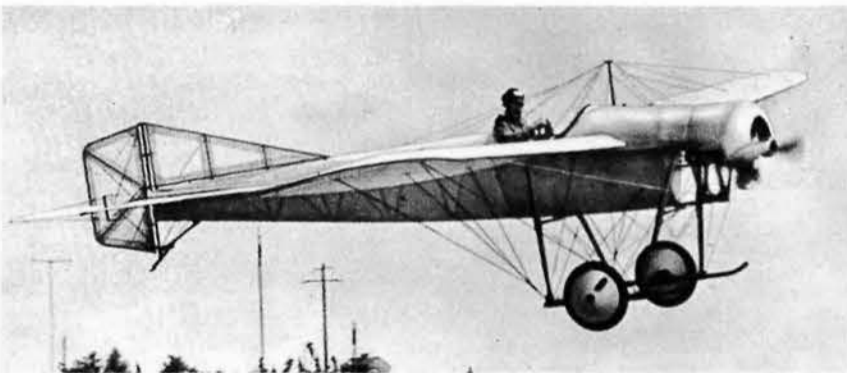
Above: The 1912 Blackburn single-seat monoplane with 50 hp Gnome rotary engine, seen flying post-WW2, is still going strong with Shuttleworth at Old Warden. See 22.9.49 above. (via Jack Meaden)
