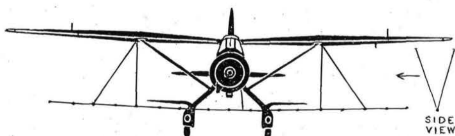
Below: Ex-RCAF Lysanders were fitted with specially designed low-slung spray bars for crop spraying in Canada: see 12.11.48. (Jack Meaden)
