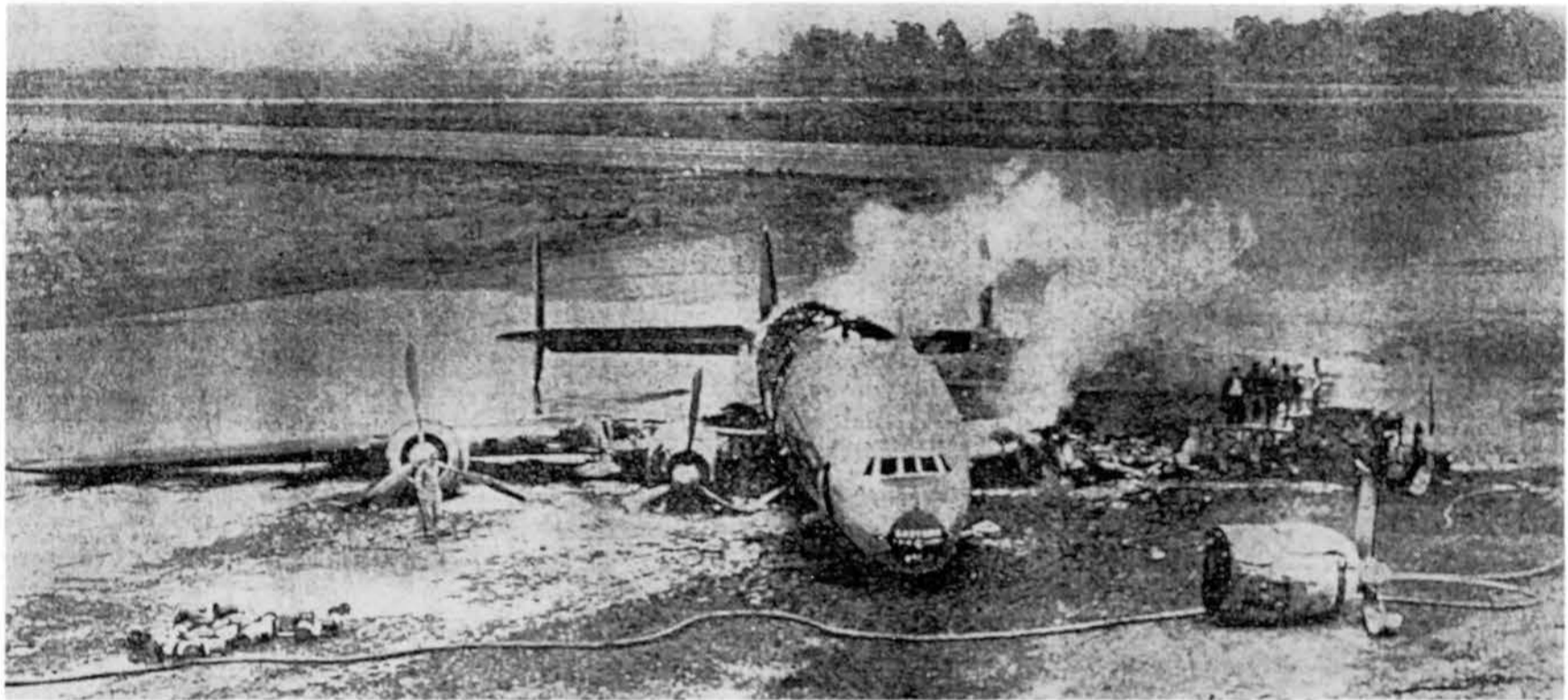
Above: The smouldering wreckage of Super Constellation N6214C at McChord Air Force Base on 6.9.53. The port engines are completely detached, the fuselage burnt out and the firefighters still in attendance. (via John Wegg)
