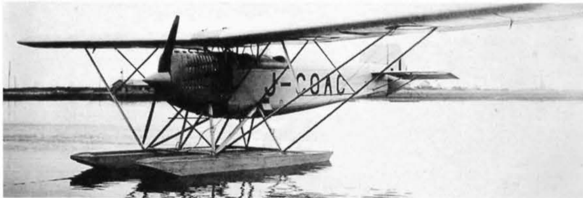
Left: J-COAC was a Kawanishi K-8A parasol-wing monoplane, one of five floatplanes used by NKKK as long-range mailplanes between Osaka and Fukuoka following the success of the K-7A.
