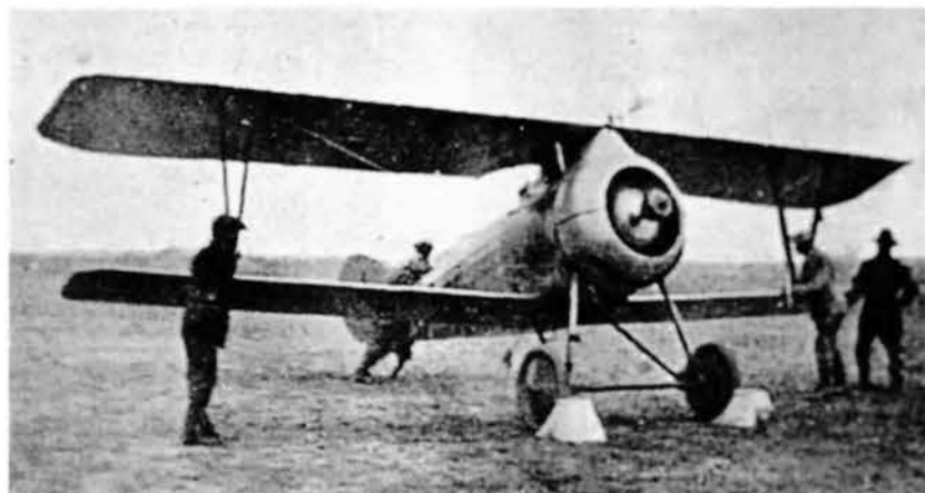
Above: Although the registration is hidden, this Nieuport 24/Ko 3 civil conversion has an additional fuel tank under the centre section and was used in the Tokyo - Osaka mail competition in November 1922.
