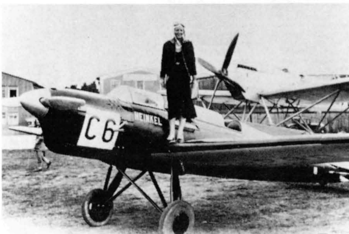
Top: Messerschmitt M29 D-2309 with Rundflug number B4, showing the high-mounted tailplane that failed with fatal consequences on two aircraft.
