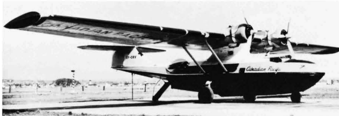
Left: Boeing of Canada-built PBY-5A Canso CF-CRV was acquired by Canadian Pacific on 8.4.46. At some stage it was converted to "Landseair" standard as shown here with modified nose profile, rear airstair and blown perspex blister window. Its fate is recorded in the entry for 11.5.53 and it was cancelled on 31.12.53. (MAP via David Legg)
