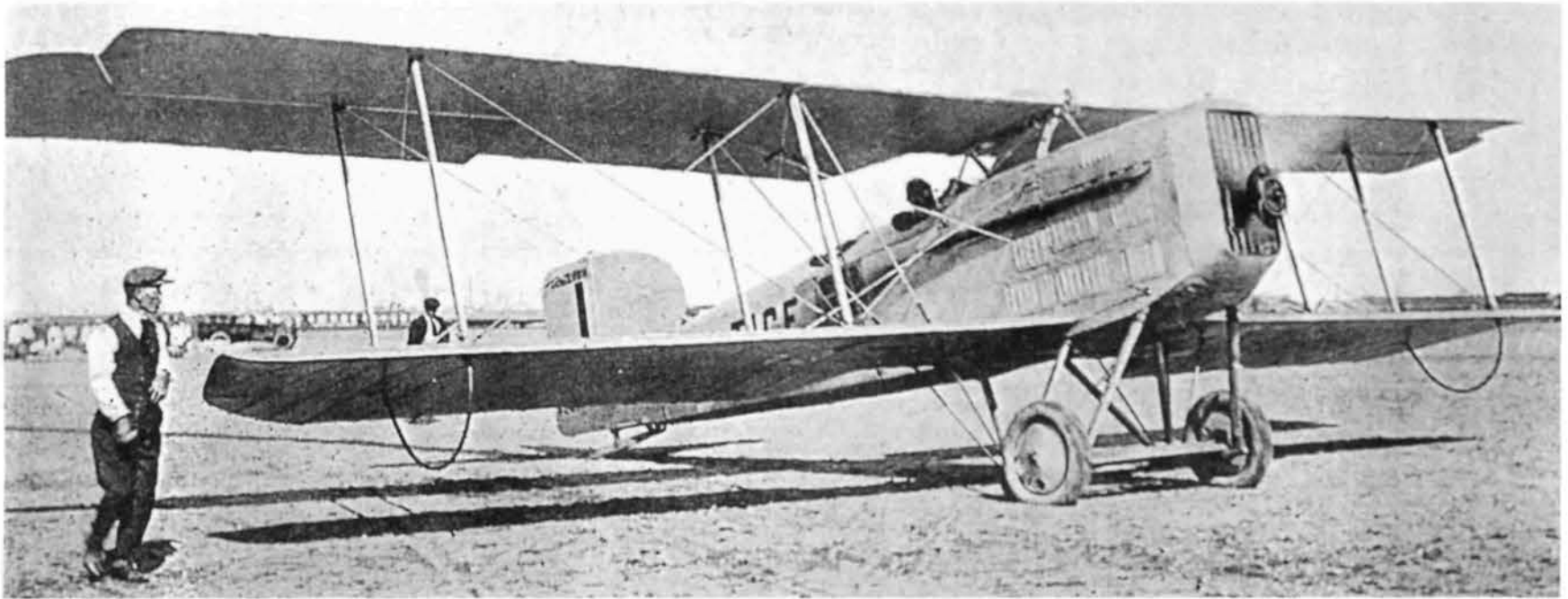
Above: J-TICE, the Nakajima B-6, was a licence-built Breguet Br 14 with a Rolls-Royce Eagle engine. Left: J-TILO, the Fukunaga Tenryu 10, was entered in a competition 6.23 with a 500 litre (110 gal) fuel tank in the cabin in place of the 4 passenger seats. Far left: J-TIOR, the Shirato 40 2-seat trainer, became a single-seater with an additional fuel tank in the front cockpit. In this form it took part in an airmail competition 11.22 but force-landed with engine trouble.
