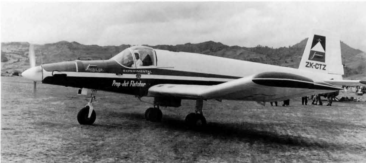
Left: The first turbine-powered Fletcher, fitted with a PT6 derated to 500 shp, was painted in James Aviation Ltd red, black and white colour scheme and inscribed "Prop-Jet Fletcher" on the nose. ZK-CTZ had a 12 inch fuselage stretch and 2 feet increase in wing span together with a strengthened structure which enabled it to 25 cwt loads, a 66% increase over the 300 hp standard FU-24. (Wim Zwakhals collection)
