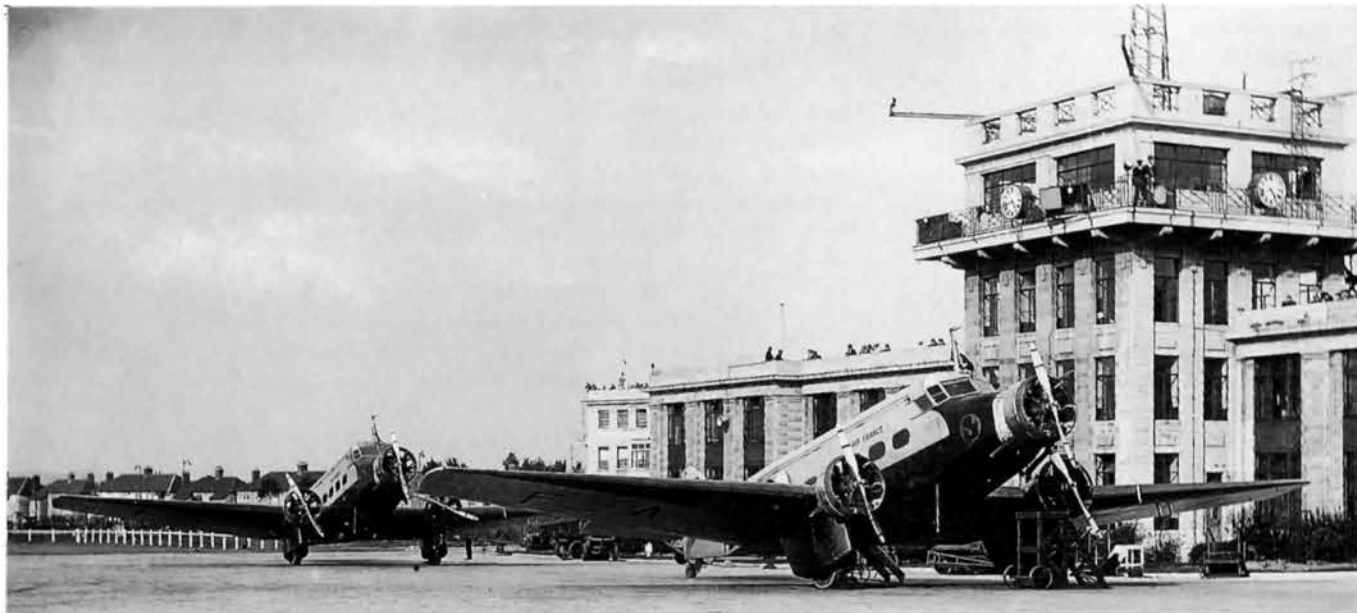
Left: Two Air France Wibault 282T-12 airliners await passenger loading outside the passenger and customs hall which formed the ground floor of the tower building. (via Jack Meaden)
