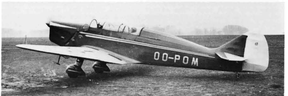
Below: Another early photo, taken at Gosselies, showing the original shallow cockpit transparencies with sliding hoods and deeper windscreen sides through which the instrument panel is just visible. On the wing is a two-piece walkway for cockpit access. (Both via Jack Meaden)
