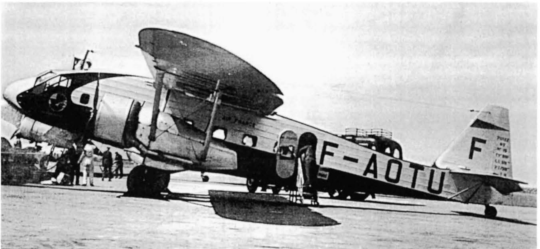
Above: Potez 620 F-AOTU "La Séduisante", whose cryptic message on 7.3.38 appears to describe a left motor problem and delayed several other flights. The 620 was the first French production airliner with a retractable undercarriage. (via Jack Meaden)
