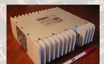
This small and light weight 5W L-To C-Band Block Up Converter is designed to be mounted on the feed horn. High power efficiency resulting in low current (<= 2 amps) consumption allows user to pass DC supply voltage via IF cable. The unit is ideal for network and point to point, data distribution, portable and emergency applications.
