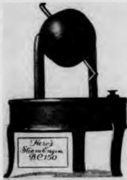
The First Steam Engine. Invented by Hero the Greek in 150 B.C.
