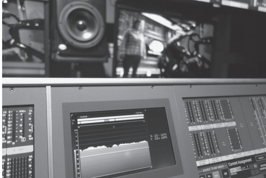
FIGURE 5.14-13 A contemporary audio console displaying a loudness histogram and an LKFS target value during content creation.
