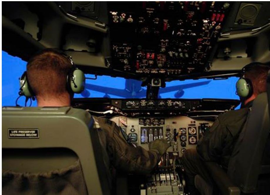
Figure 8-6. High-end simulation for training air-to-air refuelling
