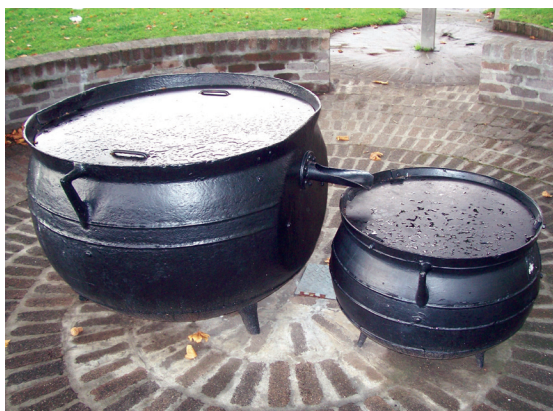
Figure 7.1. Iron 'try pots' were used to heat whale blubber to extract the oil.
