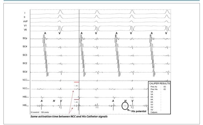
Figure 3 – Sequentially from top to bottom: peripheral derivations, coronary sinus from proximal to distal electrodes, and recording catheters close to the aortic valve and His bundle region. Similar earliest local atrial activation time is observed in relation to the onset of the P wave from the septal para-hissian region and NCC, but with no His potential seen in the later.
