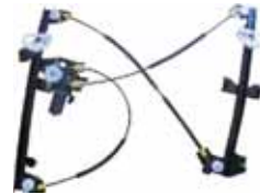
PG66-B680EL PG66-B680ER BERLINGO '96-07 FR WINDOW REGULATOR W/MOTOR 9221.G3 FL 9222.G1 FR
