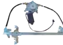
FR55-B680EL FR55-B680ER FALCON AU-BA-BF FR WINDOW REGULATOR W/MOTOR
