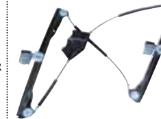
SA02-B680EQL SA02-B680EQR TOLEDO/LEON '99-05 FR WINDOW REGULATOR W/O MOTOR 1M0 837 461A FL 1M0 837 462A FR
