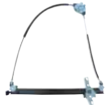
VWG1-B680AML VWG1-B680AMR CITI GLF '79-03 FR WINDOW REGULATOR MANUAL 17S 837 401D FL 17S 837 402D FR
