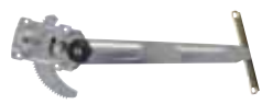
TYN2-B680BML TYN2-B680BMR HILUX RN30/40 P/UP '79-83 W/VENT FR WINDOW REGULAOTR MANUAL 69802-89106 FL 69801-89106 FR
