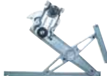
TYE10-B680ML TYE10-B680MR CROLLA/RUNX EARLY '02 FR WINDOW REGULATOR MANUAL 69820-02200 FL 69810-02200 FR
