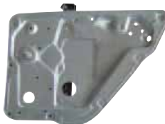
SDB1-B681ML SDB1-B681MR FABIA '00-06 RE WINDOW REGULATOR MANUAL 6Y0 839 655 RL 6Y0 839 656 RR
