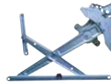
TYN20-B680EQL TYN20-B680EQR TACOMA '95-04 FR WINDOW REGULATOR W/O MOTOR 69802-35090 FL 69801-35100 FR
