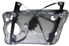
SDB1-B680EQL SDB1-B680EQR FABIA '00-06 FR WINDOW REGULATOR W/O MOTOR 6Y1 837 461 FL 6Y1 837 462 FR
