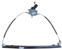
RN42-B680EL RN42-B680ER MEGANE SCENIC '96-03 FR WINDOW REGULATOR W/MOTOR 7700 838 592 FL 7700 838 591 FR
