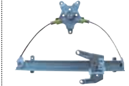
NSB6-B681AML NSB6-B681AMR SENTRA B13 '90-94 RE WINDOW REGULATOR MANUAL 82701-50Y05 RL 82700-50Y05 RR
