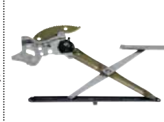
TYN4-B680CEL TYN4-B680CER 4 RUNNER '90-95 4D W/O VENT FR WINDOW REGULAOTR W/MOTOR 69802-35040 FL 69801-35040 FR
