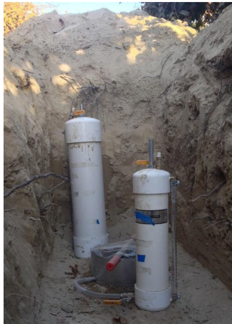
Figure 1 Infiltration Test with a Dual-ring Infiltrimeter and Mariotte Bottles. Pre- and post-nitrate concentrations were measured and plugged into HYDRUS 1D model to assess immobile zone nitrate capturing potential.
