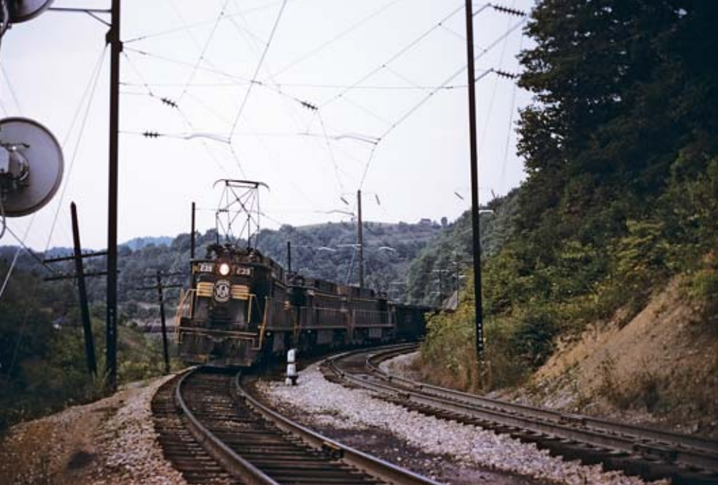
Three GE-built EL-C electrics lead a Virginian coal train east near Clarks Gap, W.Va., on Sept. 9, 1960. Built in 1956-57, the EL-Cs outlived Virginian's electrification. Harold Cavanaugh
