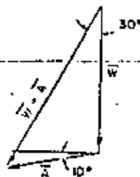
(b) Vertical Plane Oriented S 45^\circ W Containing Vectors \bar{W} and \bar{A}
