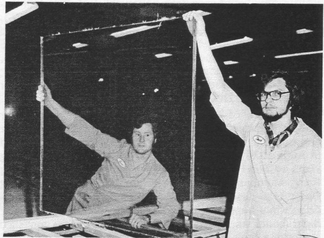
Mr. Dave Geibel, left, General Electric Tech representative, inspects a completed window. While this window is tinted or colored bronze, it is also available in clear and gray. This is the only all-plastic window currently "listed" by the Underwriter's Laboratories as meeting U.L. 752 Class III, the laboratory's standard for bullet resistant glazing (windows) tested for protection from .44 Magnum Super Power small arms.
