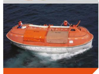
These boats are built to comply with the latest SOLAS amendments, and designed to be launched using Pivot Gravity, Gravity Roller Track Davits, Hydraulic Stored Power Davits and Platform Davits.
