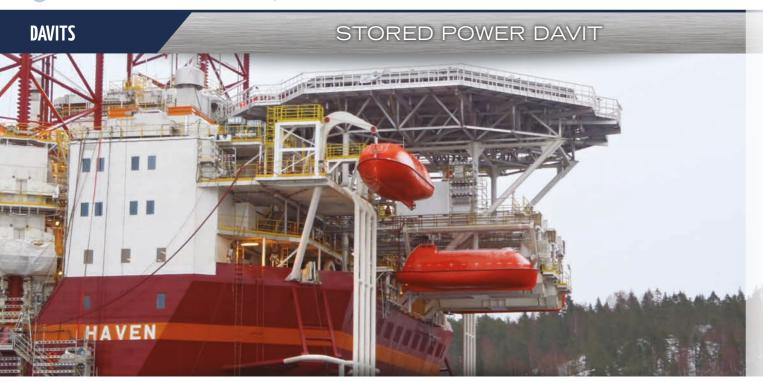
Our Stored Power Davit is designed to offer a compact solution for the safe and efficient launch and retrieval of lifeboats and rescue boats. It is built for long term, reliable operation in a harsh and hazardous marine and offshore environment.
