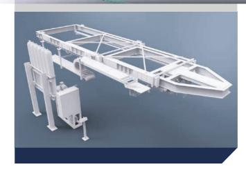
Our OVERHEAD DAVIT series for launch and retrieval of lifeboats and rescue boats are designed for long-term reliable operation. even in the severest corrosive marine environment.
