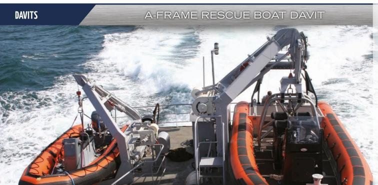
A-FRAME DAVITS have been designed to be as lightweight and compact as possible. Our equipment is designed for long-term operation under the severest and most extreme conditions, in a highly corrosive marine environment.
