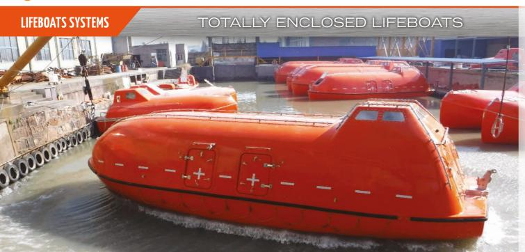
ACEBI's Totally-Enclosed Lifeboats are designed and tested to comply with the latest IMO / SOLAS regulations (MED 96/98 EC). Two versions are available: tanker and conventional. Two conventional boat models are available: PELB (Partially-Enclosed Lifeboats) and TELB (Totally-Enclosed Lifeboats).
