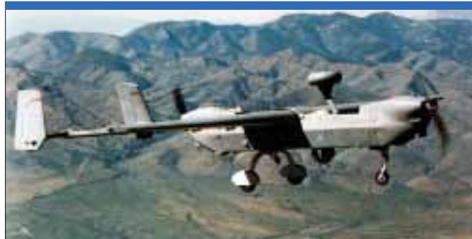
The baseline twin-engined Northrop Grumman RQ-5A Hunter traces its origins back to the IAI Impact project. At least 56 have been purchased by the US Army. (Northrop Grumman)
