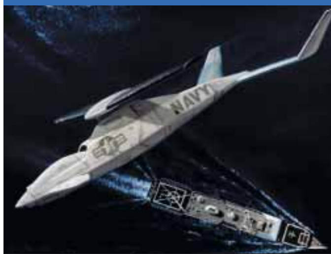
The Boeing X-50 Dragonfly canard rotor/wing technology demonstrator will investigate the feasibility of a high-speed operational drone using the stopped-rotor concept. (Boeing)
