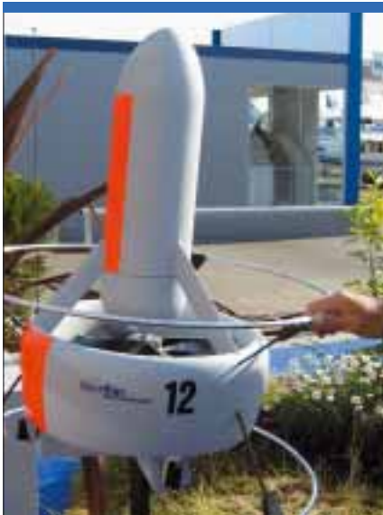
Sagem unveiled its Bertin-based electrically powered Odin at the 2005 Paris Air Show. (Armada/EHB)
