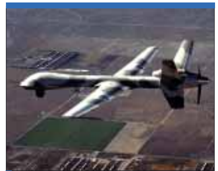
The Predator-B is easily distinguished by its tail configuration. The centreline ventral fin of the -A is retained but the main surfaces are moved above the fuselage. (General Atomics)
