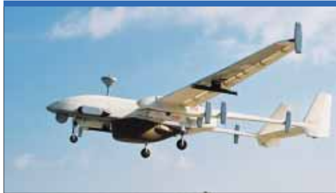
IAI Heron in multi-sensor configuration, with maritime search radar, a small side-looking radar array, two jammer pods, a multiplicity of elint antennas, an EO/IR ball and satcom tower. (IAI)
