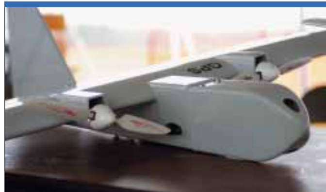
Like the Desert Hawk, the AeroVironment Dragon Eye is bungee-launched. The US Marine Corps plans to procure 342 three-drone systems under a five-year programme. (US Navy)
