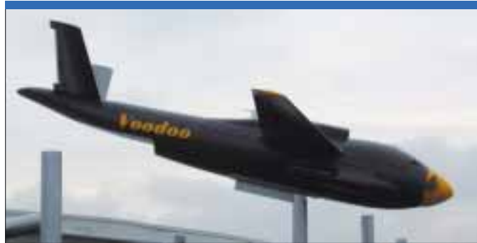
There remains a strong market for target drones for short-range air defences, as exemplified by this Meggitt Defence Systems Voodoo, a 210-kg vehicle with a 108-kW engine. (Armada/EHB)
