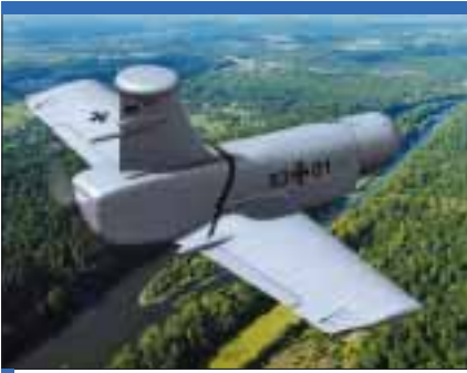
The German Army's KZO is produced by Rheinmetall Defence Electronics and is designed for stealthy day/night all-weather operation, with de-icing provisions. (Rheinmetall)
