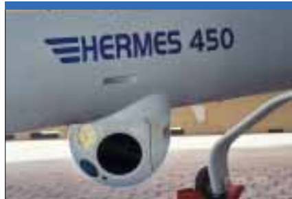
The Compass family includes payloads equipped with a third-generation Flir, eyesafe laser rangefinder/diode pumped advanced designator, and night vision goggle-compatible laser target illuminator. (Elbit)
