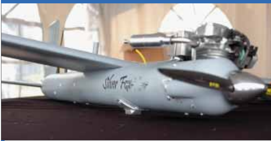
The Advanced Ceramics Research Silver Fox is a 12.2-kg modular drone burning mogas or avtur fuel. It is used by the US Marine Corps in Iraq and is being evaluated by the Canadian Forces. (US Navy)
