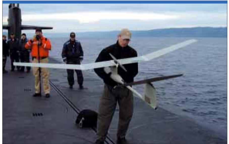
AeroVironment Pointers are used by the US Air Force, Army and Marines. Here Air Force airmen from the 22nd and 23rd Tactics Squadrons are trialling use from an Ohio-class submarine. (US Navy)
