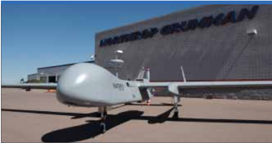
Unlike earlier Hunters, the Hunter II is single-engined. It makes extensive use of structural components from the IAI Heron for enhanced endurance and ceiling. (Northrop Grumman)
