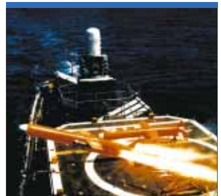
Northrop Grumman has manufactured over 7500 examples of the BQM/MQM-74 target drone series. The straight-wing BQM-74E is now being superseded by the swept-wing BQM-74F. (Northrop Grumman)
