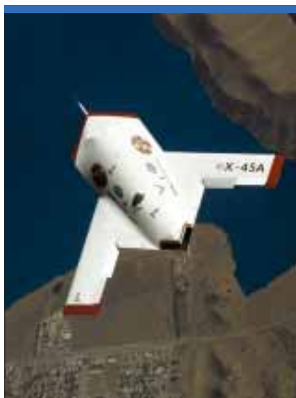
The planform of the Boeing X-45A is a typical configuration designed for radar stealth, with leading and trailing edges aligned to produce two narrow response spikes. (Nasa)
