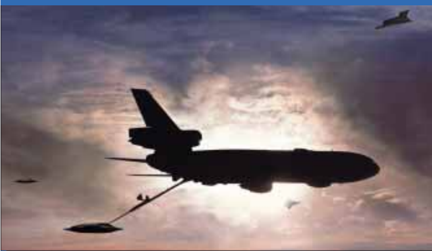
The way ahead? Future combat drones will require in-flight refuelling. In this impression, a receptacle-equipped J-Ucas can be seen taking fuel from the boom of a KC-10A. (Northrop Grumman)
