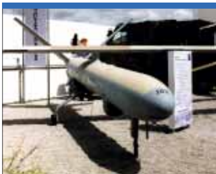
The Thales Watchkeeper WK450 is basically an Elbit Hermes 450 drone equipped with a Thales I-Master radar and an Elop Compas IV EO/IR sensor. (Armada/RB)
