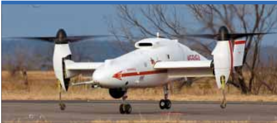
Tilt-rotor technology from the XV-15 and V-22 series is now being applied to drones. The first full-scale Bell TR918 Eagle Eye began hover trials in January 2006. (Bell)
