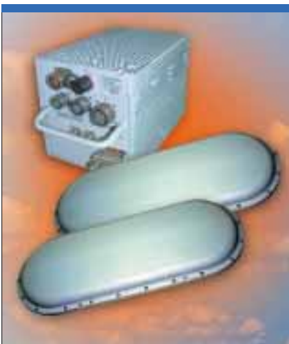
The Elisra AES-210/V elint and electronic support measures package weighs less than 22 kilos, operates in the 1 to 18 GHz band and has an RS422 interface. It uses interferometer and differential Doppler to provide fine direction finding. (Elisra)
