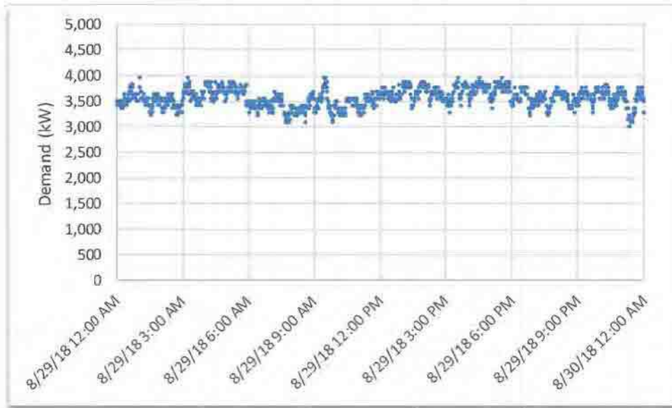
Figure 15 – 8-29-18 Electric Demand – Highest Production Day (daily values of 139 tons production and 85,736 kWh electric usage)
