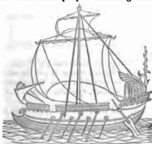
On the middle of the ship was erected the mast (*MALUS*), which was raised<sup>6</sup> when the ship left the harbour, and taken down<sup>7</sup> when it approached the land; the place where it stood was called *MODIUS*.<sup>8</sup> The ships of the ancients had only one mast.
