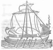
On the middle of the ship was erected the mast (MALUS), which was raised 6 when the ship left the harbour, and taken down 7 when it approached the land; the place where it stood was called modius.8 The ships of the ancients had only one mast.
