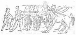
TME above cut, taken from a picture in one of the romes of a wine shop, lately excavated at Pompeli, represents a wine-cart, and shows the way of filling the amphoras. The clumpy transverse yoke by which the horeas are fastened to the pole is worth attention. We have also to point out the large skin, occupying the whole of the waggen, and supported by a frame-
