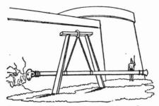
(ARIRS), a long beam, like the mast of a ship, and armed at one end with iron in the form of a ram's head; whence it had its name. It was suspended by the middle with ropes or chains fastened to a beam that lay across two posts, and hanging thus equally balanced, it was by a hundred men, more or less (who were frequently changed), violently thrust forward, drawn back, and again pushed forward, till, by repeated strokes, it had shaken and broken down the wall with its iron head.9
