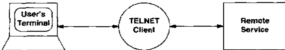
Figure 25.1 Conceptual role of a TELNET client. The client must transfer characters from the user's keyboard to a remote service, and it must transfer characters from the remote service to the user's display.
