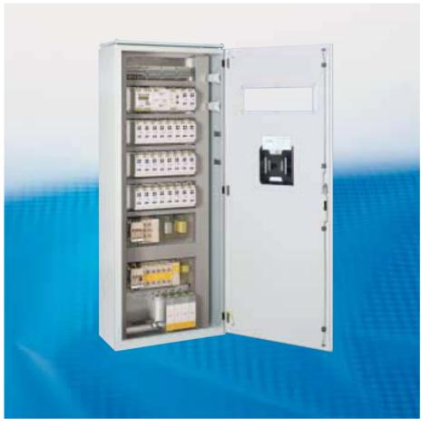
As well as providing a dependable supply of power (230V AC/220 V DC) to safety and exit luminaires, the ZB-S automatically tests the system and individually monitors each CG-S luminaire (up to 20 per circuit), and it does all this using the power supply cable alone.
