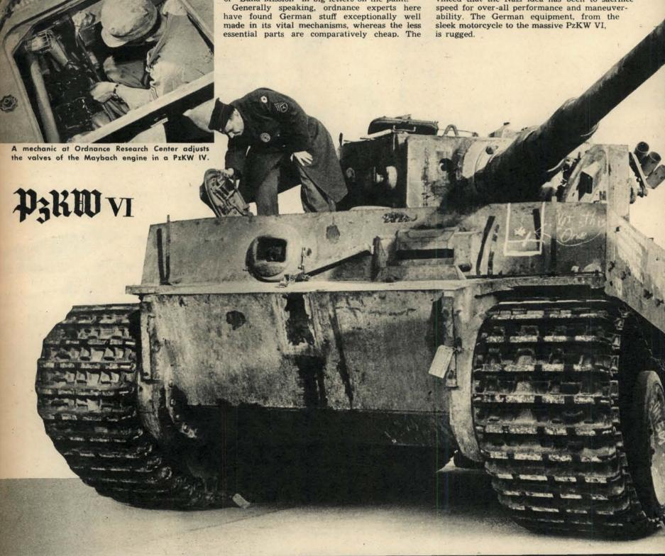
This is the famous Tiger (with a picture of its namesake painted on the face plate), the largest and heaviest German tank. Weighing 6112 tons, it is propelled at a speed of from 15 to 18 miles an hour by a 600-to-650 horse-power Maybach V-12 cylinder engine. Maybach engines are used in many of the Nazi panzer wagonen and in submarines. The PZKW VI has an armor
