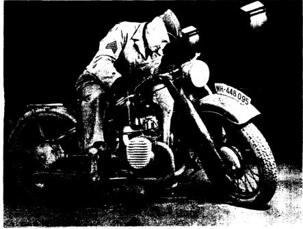
The Nazi BMW motorcycle has an opposed horizontal twin engine, driving the rear wheel by a shaft instead of a chain. Unlike most European models it has a hand gear shift similar to conventional U. S. models.
