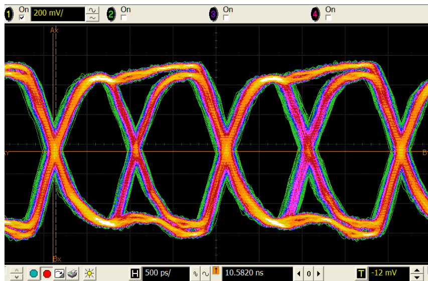
FIGURE 6.11: Eye diagram for the voltage mode driver at receiver input.
