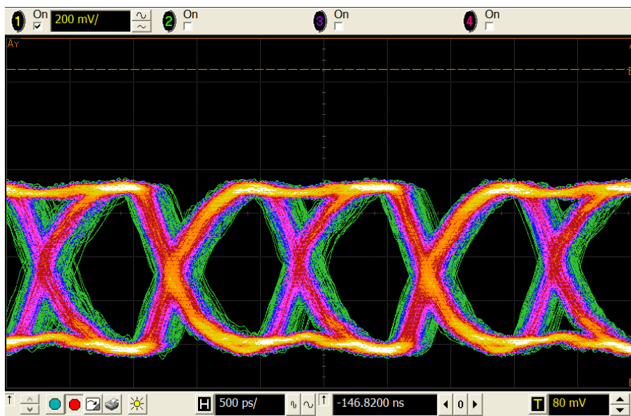
FIGURE 5.16: Eye diagram for the current-mode driver at receiver input.
