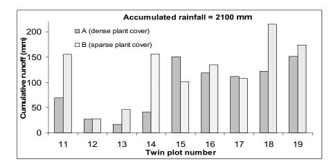
Fig 5.- Accumulated runoff (from Sept 91 to Aug 2000) along the catena, from lower ( $n^{\circ}$  11) to upper hillslope ( $n^{\circ}$  19). A and B are twin runoff-erosion plots as shown in Fig 2.
