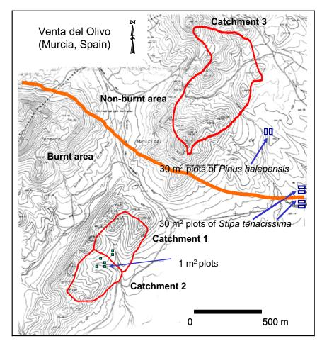
Figure 8. Experimental set-up at El Picarcho catchments (Source: Gómez-Plaza, 2000).
