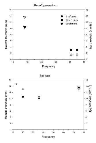
Figure 10. Threshold of rainfall depth and rainfall intensity to generate runoff (Grey filling: rainfall intensity threshold; black filling: rainfall depth threshold) (Source: Boix-Fayos et al., submitted).
