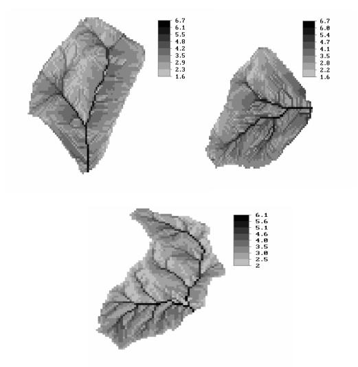
Figure 13. Topographic indices for catchment 1 and 2 (above, factors aspect, contribution area and slope were used) and topographic index for catchment 3 (below, factors aspect and contribution area were used) (Source: Gómez-Plaza et al., 2001).
