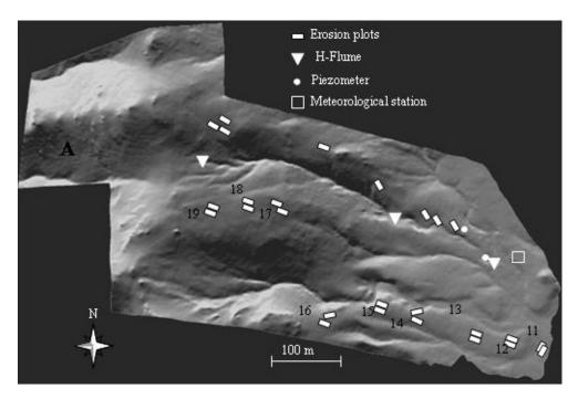
Fig 2.- Rambla Honda field site (map compiled from DEM at 1 m resolution), showing runoff-erosion plots, runoff gauges in the catchment and meteorological station.
