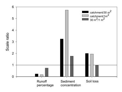
Figure 9. Scale ratios for runoff percentages, sediment concentration and soil loss for 1999 and 2003. Observe that larger areas have higher values of soil loss and sediment concentration compared to smaller areas (values above reference line 1) and larger areas have lower runoff coefficients than smaller areas (values below reference line 1) (Source: Boix-Fayos et al., submitted).
