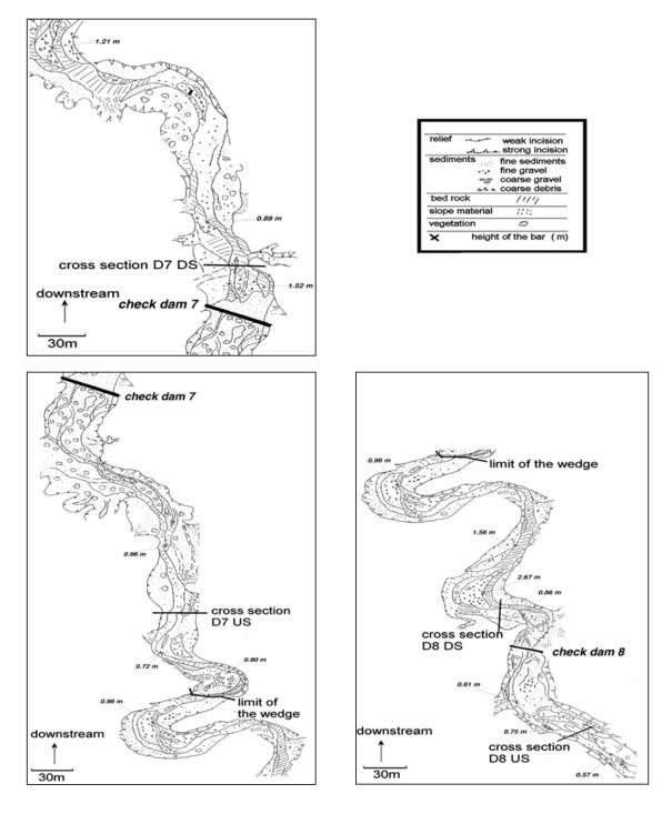
Figure 5. Geomorphological map of the stream channel in the reach between check-dams 7 and 8. The height of the bars with respect to the channel is indicated (Source: Castillo et al., submitted).
