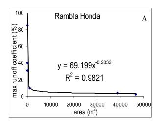
Fig 8: Relationships between catchment size and runoff coefficients.
