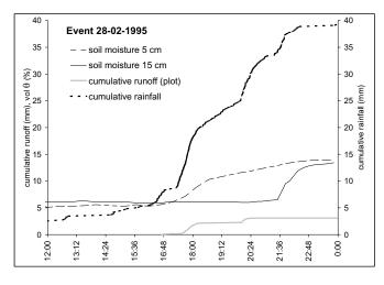
Fig 7.- Runoff by infiltration excess (Horton)
