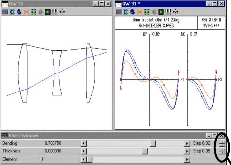
Once again, the up/down arrows on the right hand side of the slider bar window adjusts the precision and range of the sliders themselves. This demo allows the student to virtually bend the lenses of a triplet. By adjusting the sliders, the student can switch which lens is being controlled and attempt to re-balance the system aberrations by observing the ray intercept curves (a.k.a. transverse ray aberration plots).
