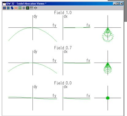
The aberration plot window shows the results of transverse ray aberration plots when third order (Seidel) aberrations are applied.
