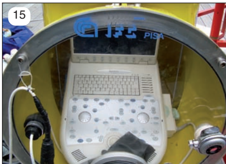
15 The Echograph in its water-tight case
