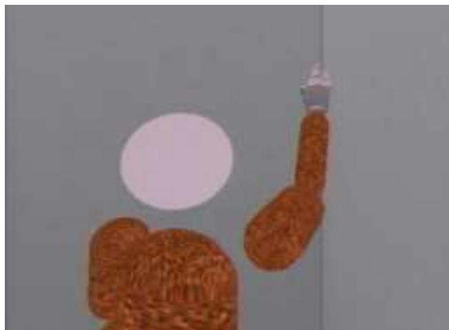
Figure 5: An articulated VR hand slides along a non-convex corner between two walls in a virtual room.
