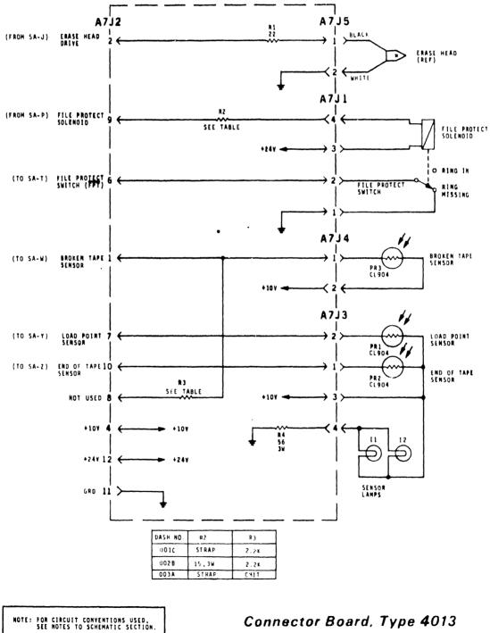
Connector Board, Type 4013 Schematic Diagram
