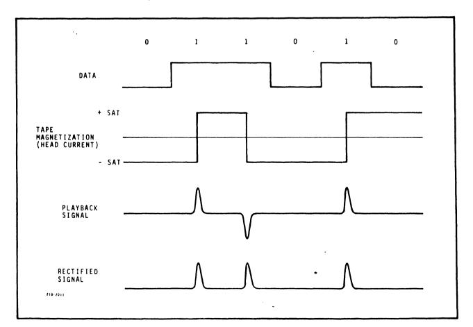
Figure 1-2. NRZ1 Waveforms - Reading
