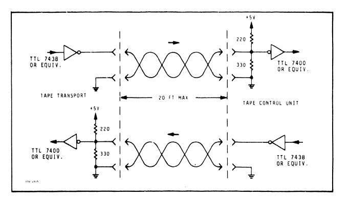
Figure 1-4. Typical Interface Configuration
