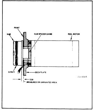
Figure 4-4. Reel Hub Assembly
