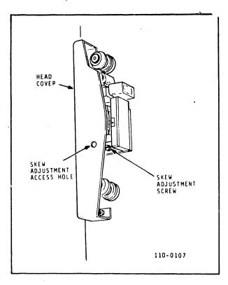
Figure 4-8. Head Skew Adjustment
