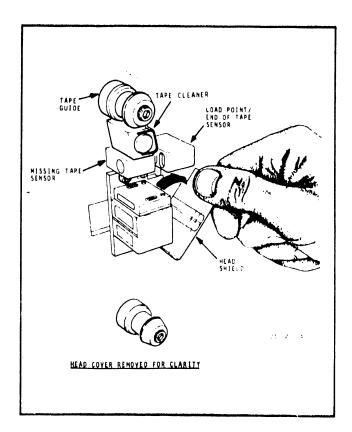
Figure 4-1. Opening of Head Shield
