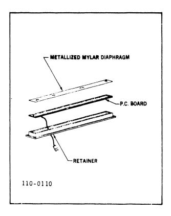
Figure 3-2. Vacuum Sensor Assembly
