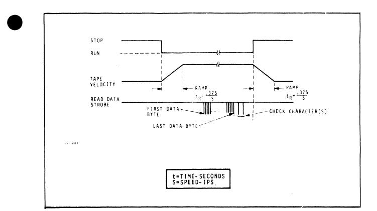
Figure 1-6. Read Forward Timing
