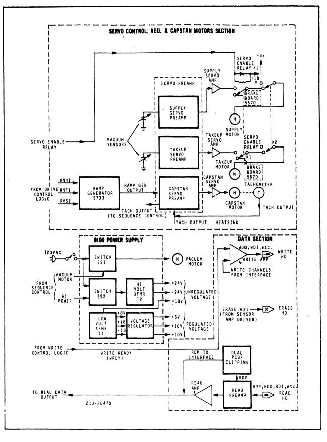
Figure 3-1. Control Logic Block Diagram
