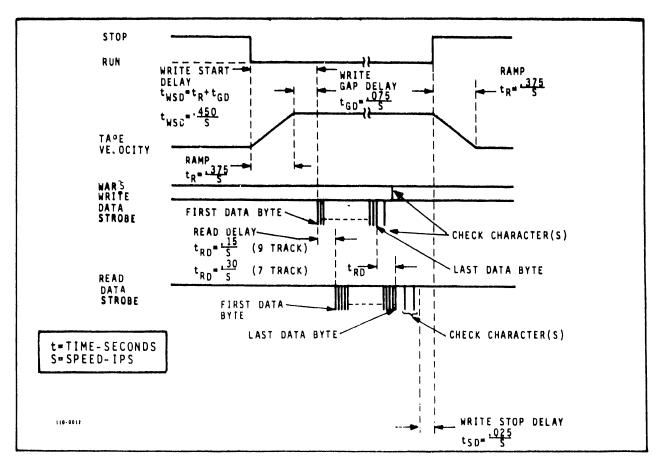
Figure 1-5. Write Timing
