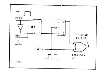
Figure 3. Write Amplifier Logic
