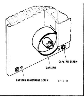
Figure 4-5. Capstan Parallelism Adjustment
