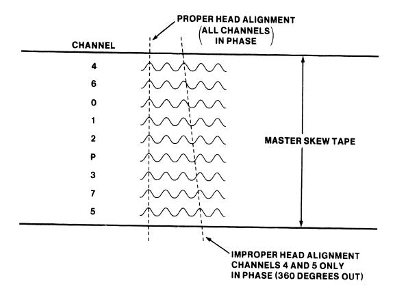
Figure 1 Read Skew Adjustment Precaution
