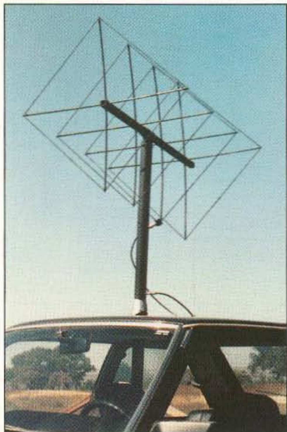
Photo A. Bob Lindsey KF5W had little hesitation about taking a big punch to the roof of the family car. He uses a commercially available quad for his 2 meter hunting.
