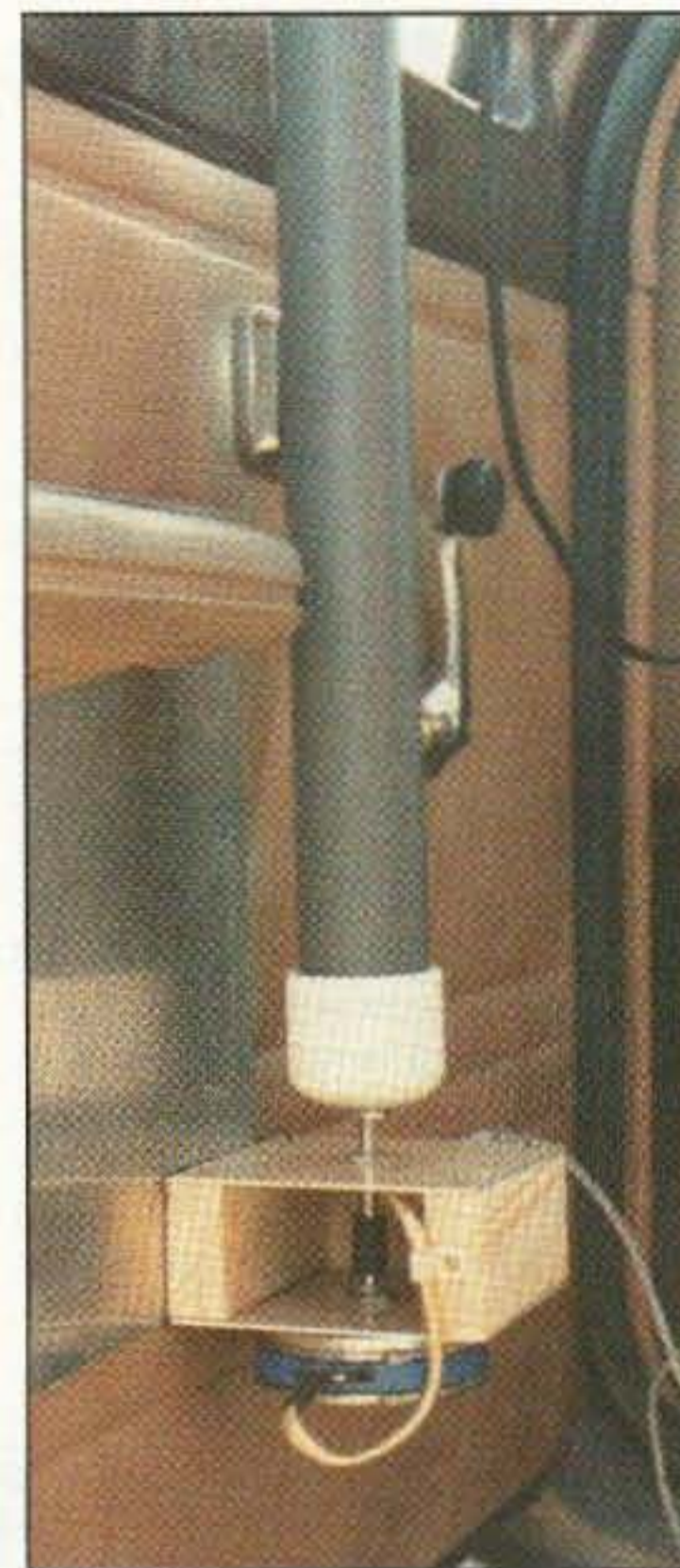
Photo C. Mount a precision 360-degree or sine-cosine potentiometer to the bottom of your antenna mast, and you can have remote indication of your mobile beam heading. Jerry Boyd WB8WFK installed his mast to the driver-side door.
