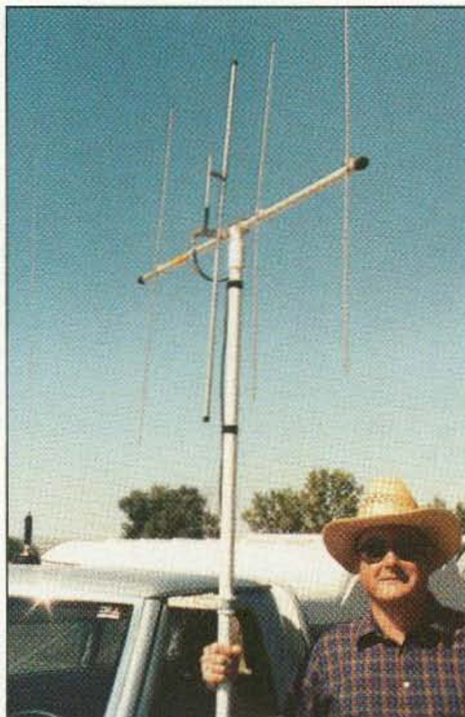
Photo B. Joe Riggs WA0TWG mounted a beam and mast to the driver's side of his pickup. Left-side overhang restrictions in your state's vehicle code may limit your antenna size using this method.
