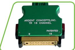
**Quick Latch** provides the same high standard of electrical performance as our Straight Mount configuration but adds the ability to mate and de-mate the TR quickly from the board by activating the red latches on either side. In a test & measurement environment, this makes the product much more user-friendly.
