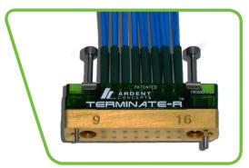
**Straight Mount** allows users to mount to a solderless footprint on your PCB with two or three screws, ensuring a reliable and repeatable connection up to 70 GHz for over 1000 mates and demates.
