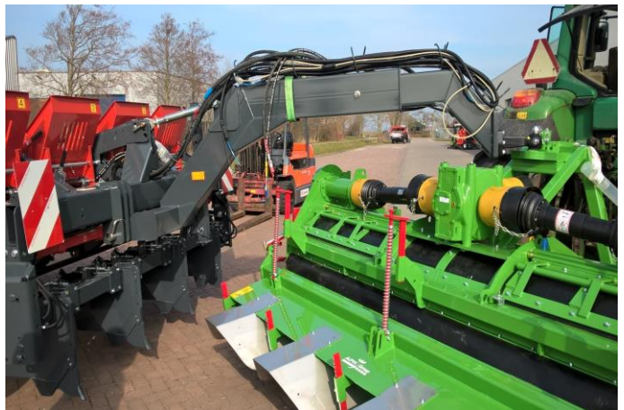
K80 connection for mounting pulled potato planter
