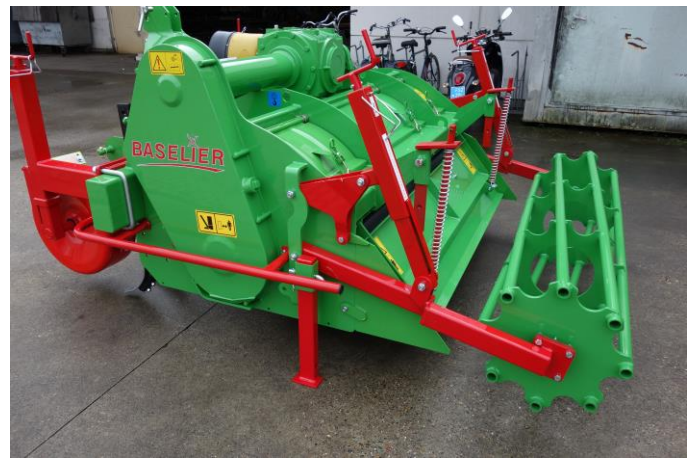
Fullwidth plate with depth roller
