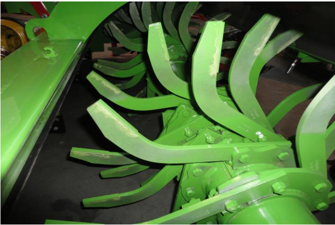
Standard hook tine mounted on hook clamp
