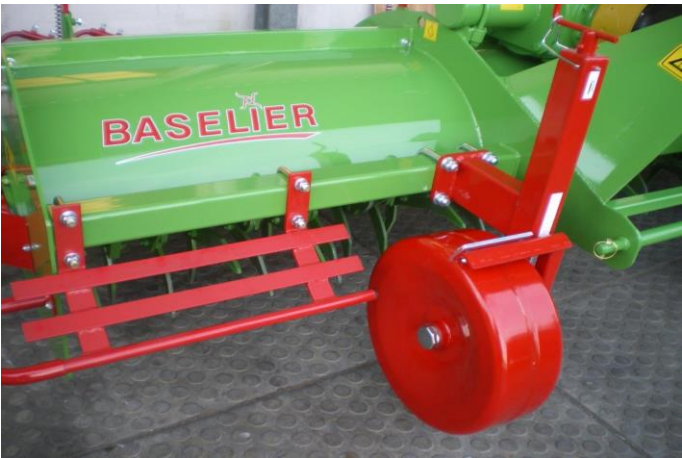
Standard steel wheel D500 x 180
