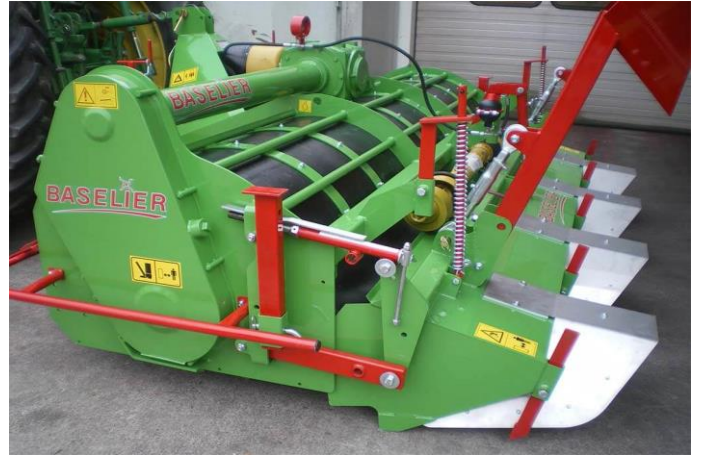
Topplate of rubber without inspection covers
