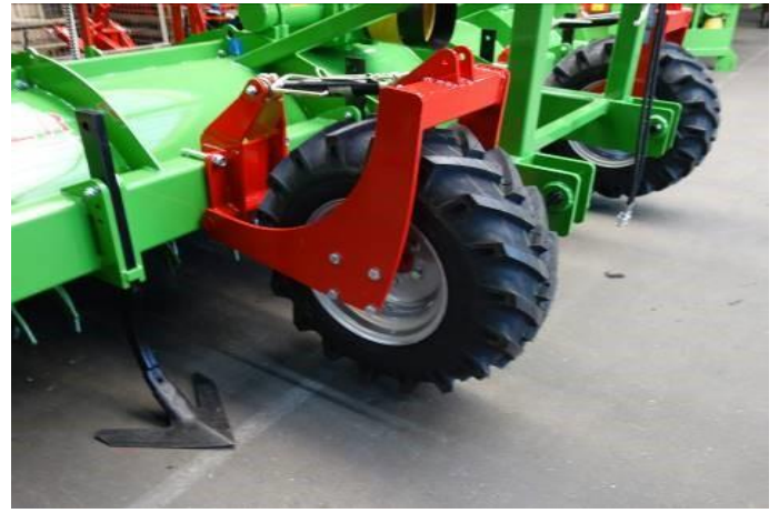
Wheel 10,0/75-15,3 with tractor profile
