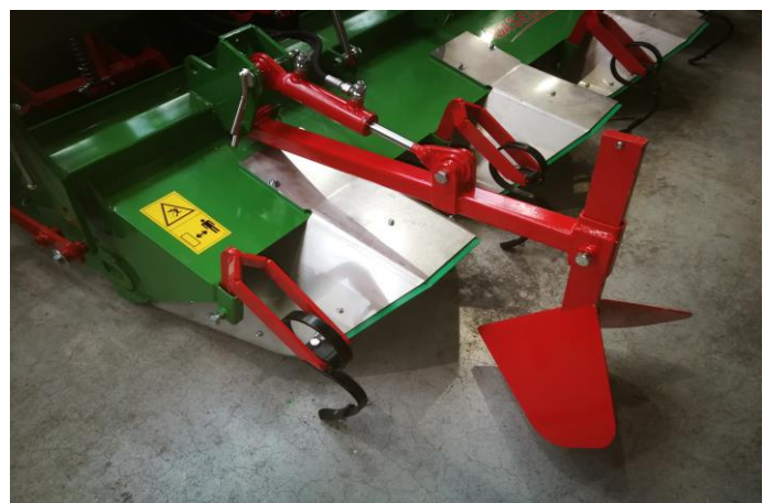
Highspeed plates with plastic, springtines in hood and hydraulic track wippers
