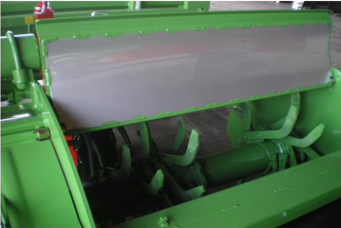
Topplate and inspection cover of stainless steel
