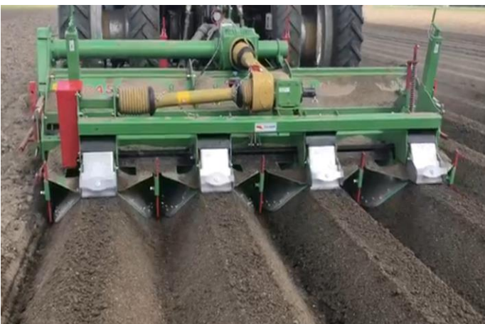
Ridginghood with 2 e rotorshaft for better crumbling of top layer for better germination of seeds
