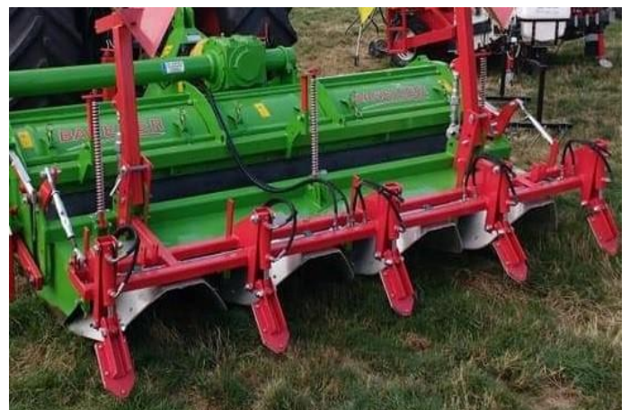
Erosionstop to prevent erosion in case of heavy rainfall
