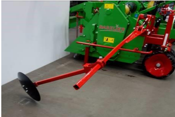
Marker with disc operated manual or hydraulic
