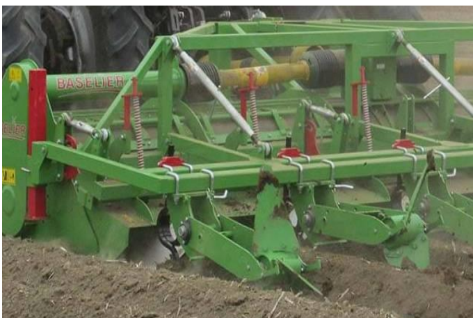
Soil blocker with spring tines and frame
