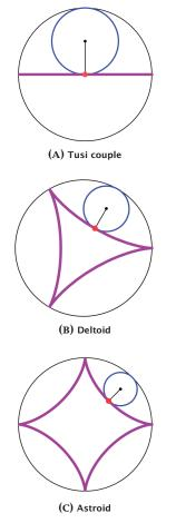
Figure 10. Circles of radius 1 trace out hypocycloids as they roll within circles of radii (from top to bottom) 2, 3, and 4.
