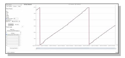
Each record of manual and automatic remitted report can be presented as trend chart or report. The report function also supports the related functions of multi-stroke display. The set report can be manually remitted to the computer as PDF or Excel (CSV) files, or automatically remitted to the PC as Excel files at regular intervals.
