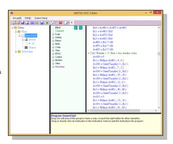
Modular design adopts text plus modular design, as long as the input conditions are simply filled in and the positions of input and output points are compared. It is not necessary to input codes as time-consuming as in the general text programming environment, nor is it like a logical ladder diagram in the form of a diagram. When the program is large, it is difficult to view the whole picture, which has the advantages of both editing forms.
