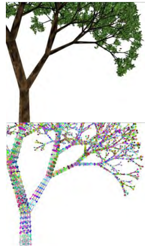
Figure 5. Result of generating particle-based model from a 3D model of a tree.
