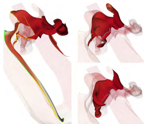
Figure 9: Pieces of stream surface extracted from the gas leak dataset. Iteratively cutting the surface with the proposed approach allows for an easy investigation of the inner areas of the vortices.
