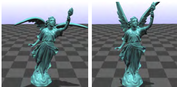
Figure 8: Left: applying external forces on the wings. Right: after releasing the external forces. Simulation rate: 116 frames per second.
