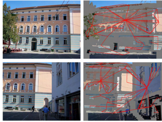
Figure 3. Building façade projected in slightly different views. Red lines (graph edges) represent spatial relationships between objects detected in the images, indicating different context in two projections for the same objects. For better overview, only some relations are visualized.
