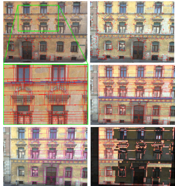
Figure 5. Top row: two examples of the same façade, matched with a sparse point cloud (red dots). Middle row: set of blocks located in each façade (left image show façade detail for better overview, right image entire facade). Bottom row: set of blocks from the first image projected into a second image and a set of transferable sites (highlighted blocks) that is derived from the projection (as sites that have no correspondence in second set).
