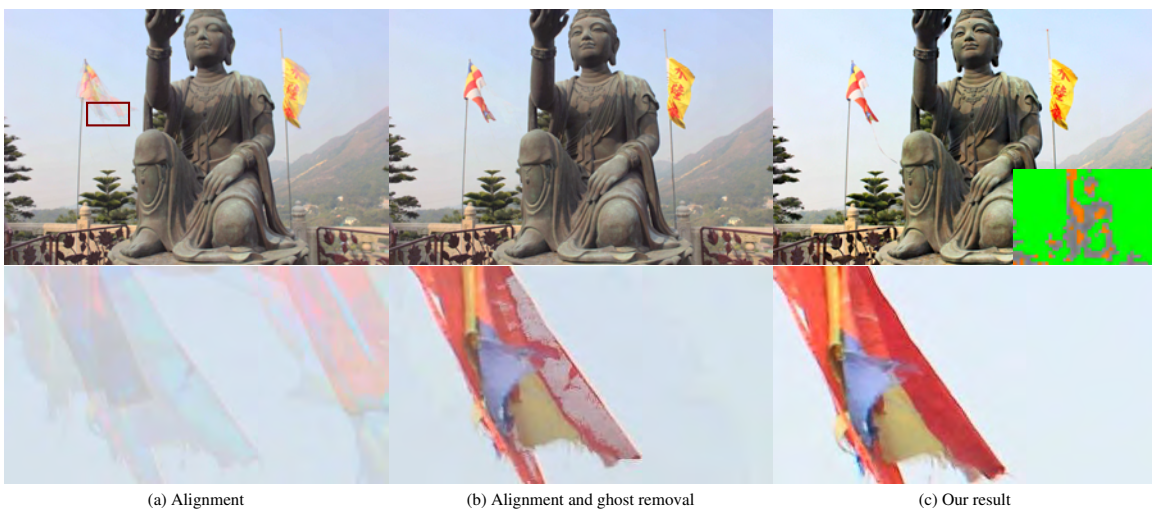
Figure 5: Left: Aligned HDR image created from hand-held exposures using the MTB algorithm. Middle: Aligned and ghost removed HDR image. Right: Our result. The insets demonstrate that ghosting artifacts are eliminated in our result. The color map shows the source exposures for different regions of the HDR image.
