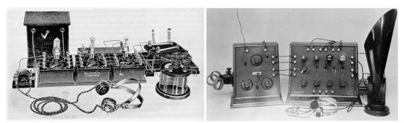
**Figure 2.11a,b: Pye "unit system" radio receiver, 1922; Burndept IV receiver, 1924 [Forty 1986]** By the mid-1920s, the radio began to enter another stage in development:
