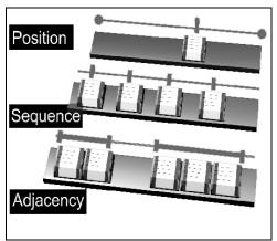
Figure 1.7: Physically structured syntax of tokens upon racks
