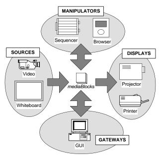
Figure 4.10: Physical interchange of mediaBlocks between supporting devices
