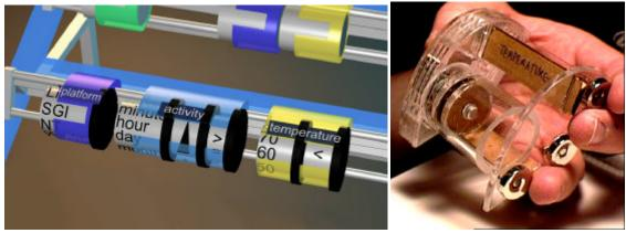
Figure 5.12: Sketch, physical prototype of second-generation parameter wheel
