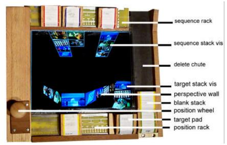
Figure 4.6: Media sequencer components
