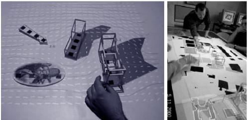
Figure 3.16a, b: "Urp" urban planning simulator [Underkoffler and Ishii 1999]
