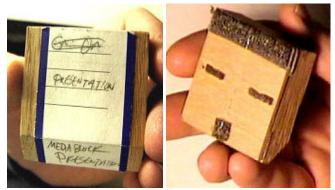
Figure 4.1: mediaBlock tokens; front, back (showing contact pads)
