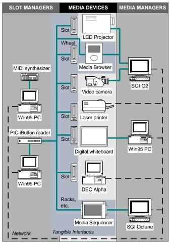
Figure 4.16: First-generation mediaBlocks system diagram
