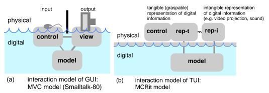
Figure 2.16a,b: GUI and TUI interaction models
