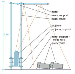
Figure 5.19: Table-based projector mirror jig
