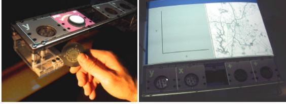
Figure 5.3: Parameter wheels and the query rack
