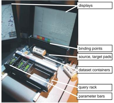
Figure 5.17: Second generation parameter bar interface
