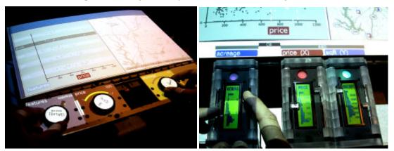
Figure 5.1: "Parameter wheels;" "parameter bars" with adjacency-based Boolean relations note: contrast adjusted on pictures throughout chapter to compensate for wide dynamic range
