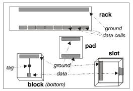
Figure 4.14: mediaBlock contact configurations
