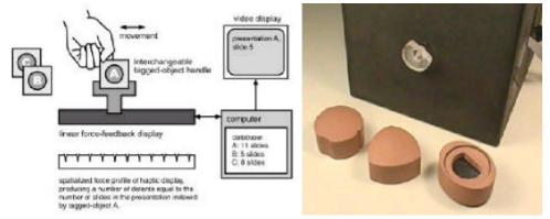
Figure 3.51: Tagged concept and prototype [Maclean et al. 2000]
