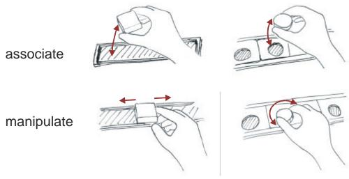
Figure 1.4: Two phases of interaction with token+constraint interfaces
