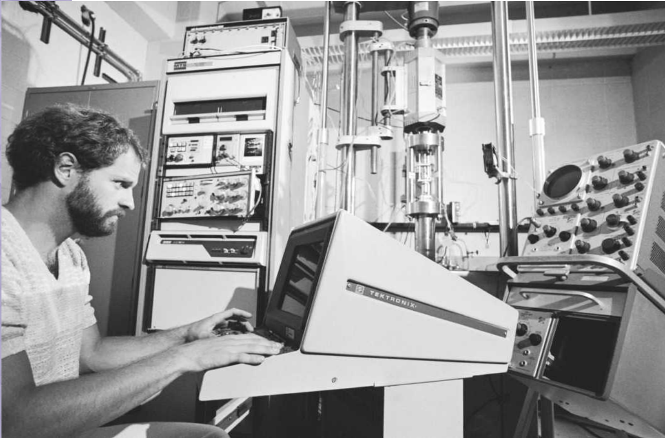
A computer user operates metallurgical testing equipment, which is controlled by a minicomputer.
