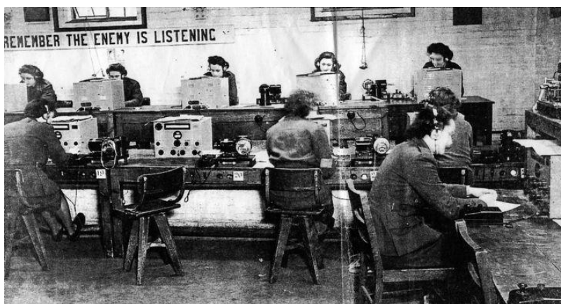
Interesting image of an intercept Set Room from WW2. Receivers believed to be the Marconi CR100. [Royal Navy had LF version, blue case, the B28] Note the Undulator which printed the Morse Characters, seen at right of each individual wireless set
