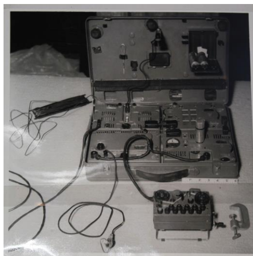
Transmitter used by Krogers at 45 Cranley Drive [Note fast keyer front, right. 140grps sent in seconds]
