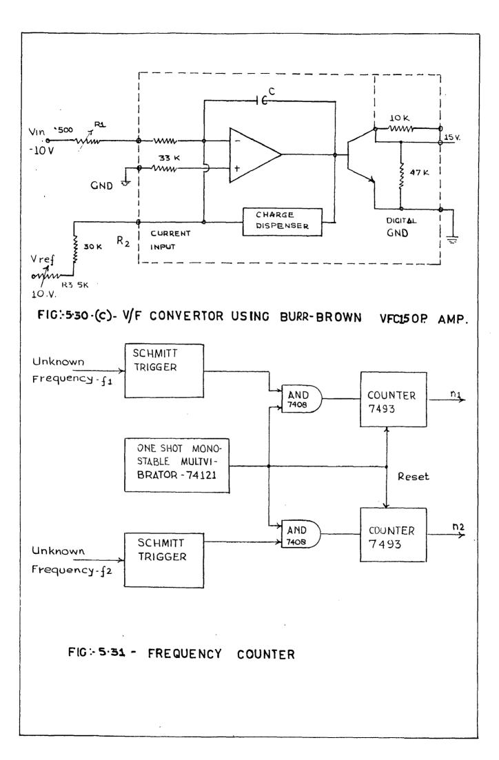
through a solutive trigger to obtain a course vave vale forme the first input to the AD gate. The second input to the AD gate is the gating pulse. If the gating pulse frequency is 1 MBs, then the counter counts the pulses in period of 10°3 exce. The gating pulse may be obtained from a astable multivibrator of Fig. 5.59(b) or from a neasefullo multivibrator.
