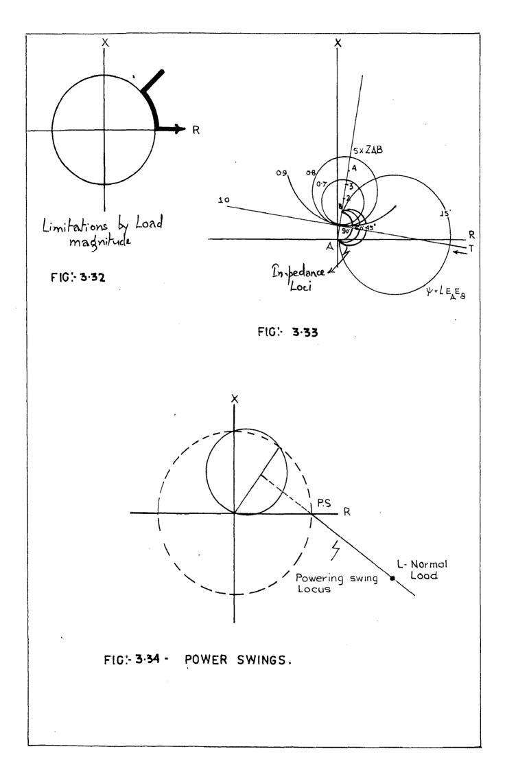
circles to the right. The relay must then be located somewhere between h and B and the impedance measured by the relay are given by the distance from that point to the circle in question. It should, however, be remembered that this impedance, but not the shape, may differ in case of changes in the network. The network condition imposing the greatest limitation in the start some should be considered.
