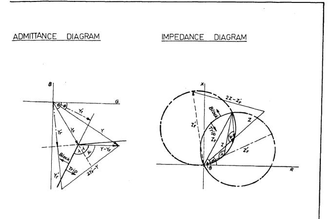
. 20(a)\_Mho RELAY WITH COMPARATOR THRESHOLD ANGLE > 90°
