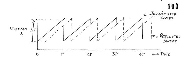
The frequency difference between the two wave forms is a constant frequency in the time interval nT + T to (n+L)Tfor  $n = 1,2,3, \dots, N$  and T is the time required for the wave to travel from the transmitter to the target and back whilst Tis the sweep duration. This constant frequency difference is stated to be directly proportional to the distance to the target and the same is given by the equation.
