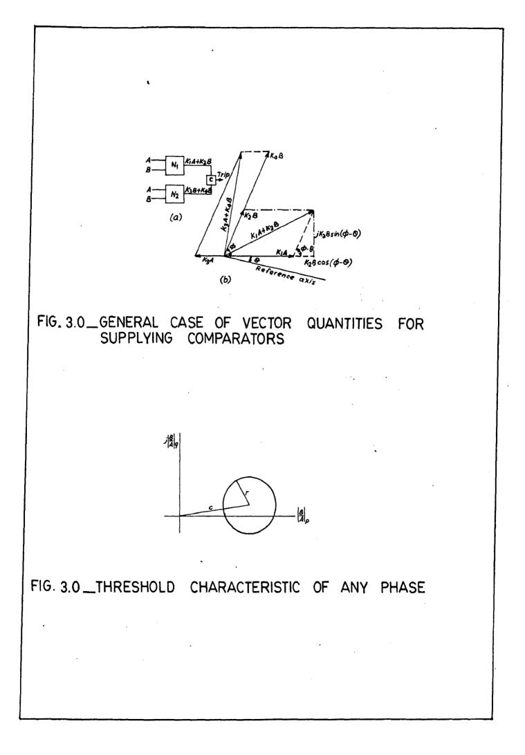
It must however be montioned that R'' is a finite quantity in single quantity relays ( level detectors) but is made substantially zero for comparators. Thus we have for distance relays the above equation to be of the form<sup>(1)</sup>
