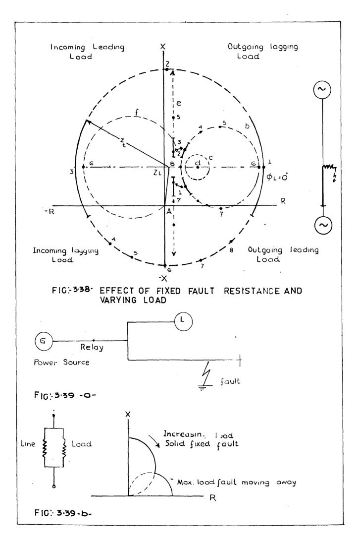
With no fault and a load of a constant magnitude but varying phase angle, the locus of the impedance seen by the relay at A is the circle 'a'. With a fault of resistance Bd and the same load condition as for 'a', the locus becomes the cicle 'b'. A smaller locus gives the locus 'c', no load gives the point 'd' Larger loads give the loci 'e' and 'f'.
