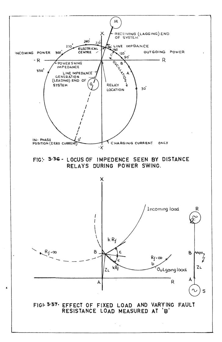
The effect of this upon the impodence seen by a distance relay is shown in the Fig. 3.35  $\propto , k \ll c$
