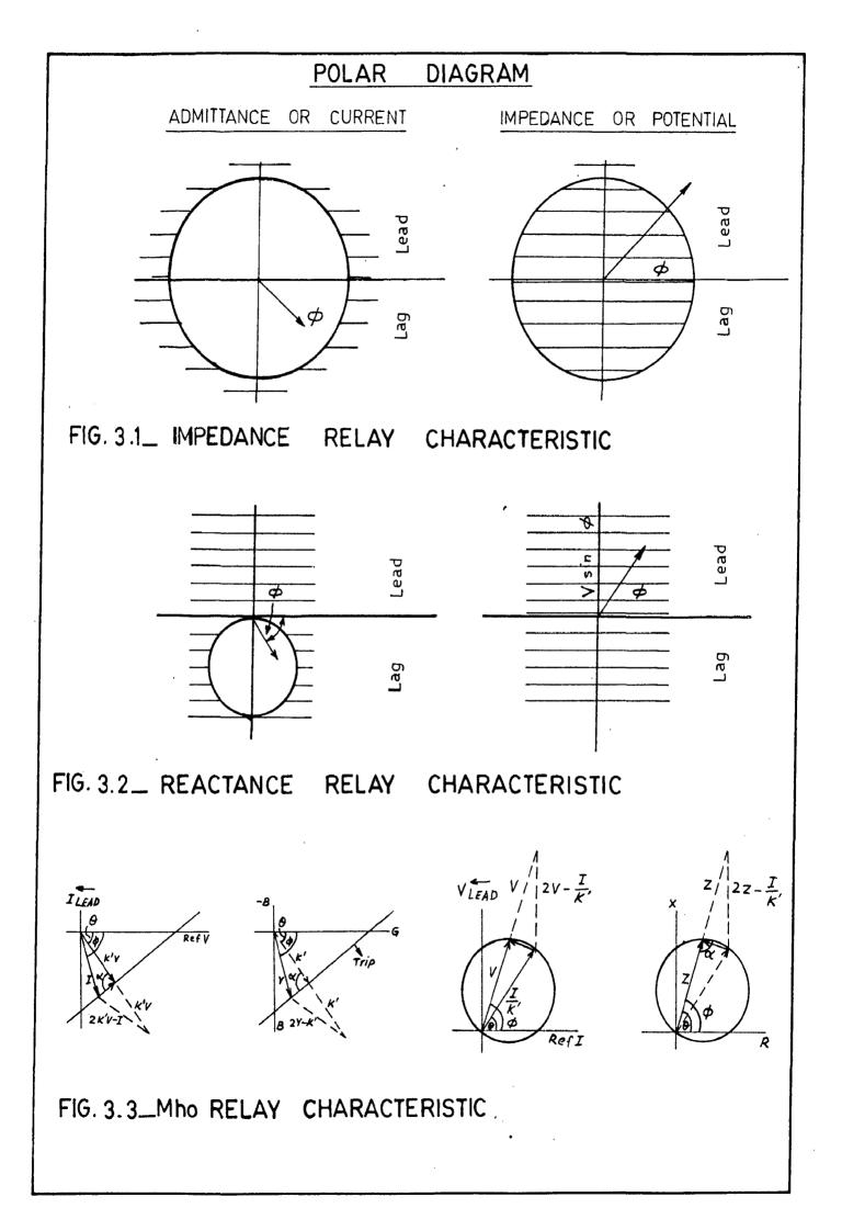
$II^{2} + VI \cos (\phi - 90) = 0$   $II^{2} - VI \sin \phi = 0$   $II = V \sin \phi$   $\frac{V \sin \phi}{I} = K$ The relay operator when  $\frac{V \sin \phi}{I} < K$ i.o. when K < K. the oblaic setting
