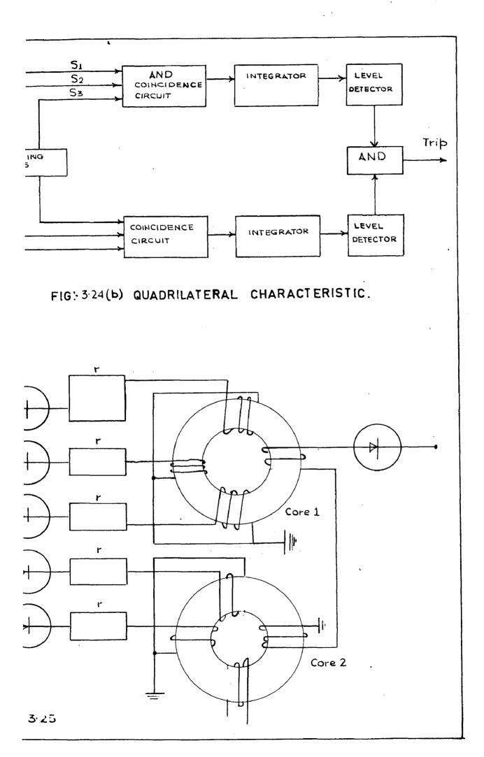
Those forrite cores claimed to be more compact, more reliable within the rated temperature, consumes less power, has no recoil, economically easy to manufacture and above all had the morit of simplicity without the requirements of any d.c. supply.
