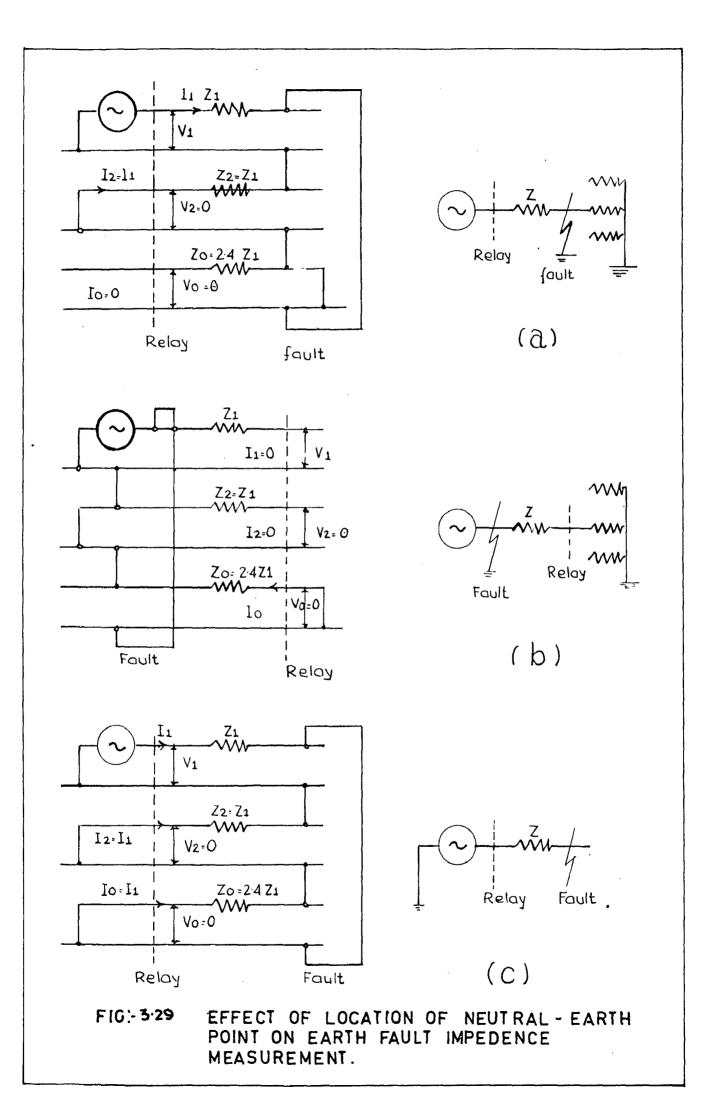
At (a) the system nontral is solidly carthod at a remote point, the source is at the relaying point and the carth fault is adjacent to the nontral-carth point, from the sequence diagram at the relay location
