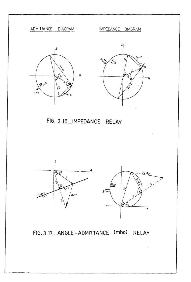
Impodence is inherently an amplitude comparison of current and voltage and the rolay trips when  $|Z| < |Z_{ge}|$  so that the impute required for an amplitude comparator are V and  $IZ_{ge}$ . The phase comparator presents contain difficulties and as such is not used in distance relays.<sup>(19)</sup>
