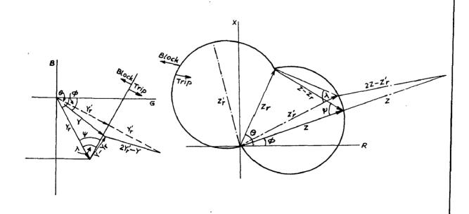
O(b) Mho RELAY WITH COMPARATOR THRESHOLD ANGLE < 90° The characteristics are plotted on both the Imp dance and Admittance diagrame as shown. Ref. Fig. 7.19.
