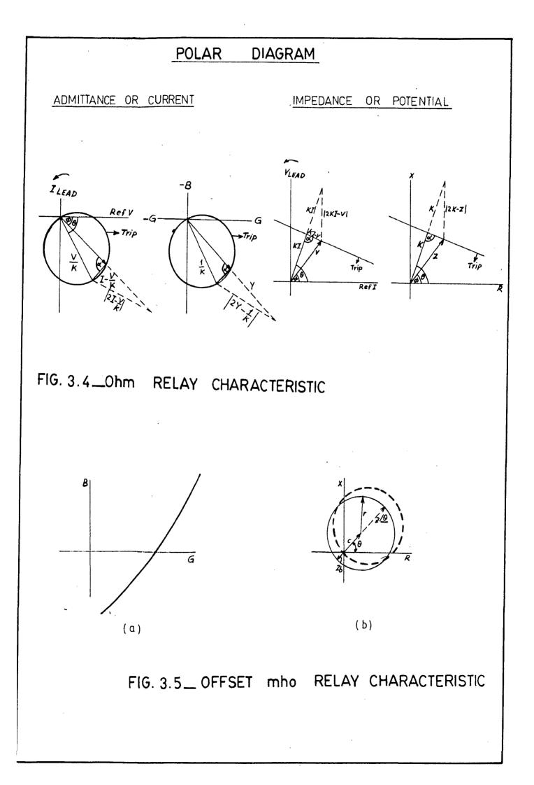
origin given by  $C = \frac{1}{2K} - \frac{1}{0}$ . The offset the relay characteristic when plotted on an Admittance diagram is again a circle but its radius and distance of the centre from the origin are inversely related to these of the circle drawn on an impedance diagram.
