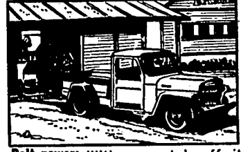
Beit power: With power take-off, it serves as a power unit for operating many types of belt-driven equipment.
