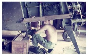
Sgt Zitzelsberger and L/Cpl Bower working on fuselage alignment. Note the creative rigging and alignment "tools" in use.
