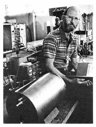
INVENTOR ED JACOBS (2352) uses his new arsenic activation neutron detector (in foreground) to count DD neutrons at 2.5 MeV. The device recently received a patent.
