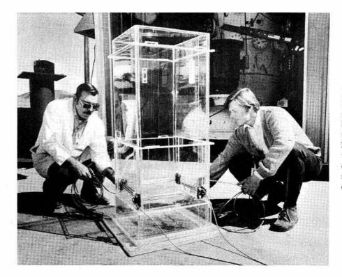
LUCITE WATER TANK is instrumented before installation in the test chamber by Paul Langdon and Dennis Mitchell (both 2514). Transparent walls of the tank permit filming of experiment with highspeed motion picture cameras.
