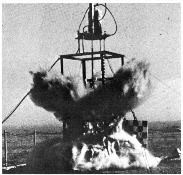
STEAM EXPLOSION results when a mass of molten iron-alumina is dropped into a tank of water. Steam explosion phenomena, part of a larger program in nuclear reactor safety, are being investigated by Dennis Mitchell (2514).
