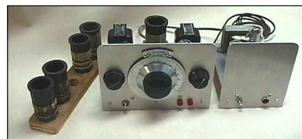
John's handsome version of the two-tube regenerative receiver with plug-in coils from How to Become a Radio Amateur .
