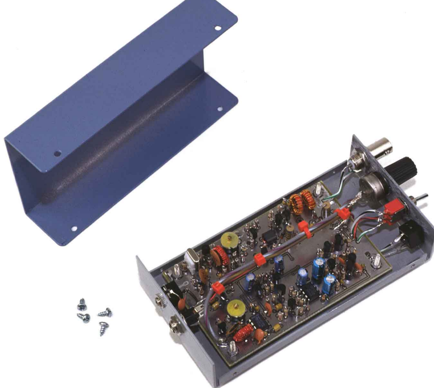
This Micromountainer is housed in an LMB enclosure. Take care to remove paint on the inside of these enclosures to ensure contact with grounded components.
