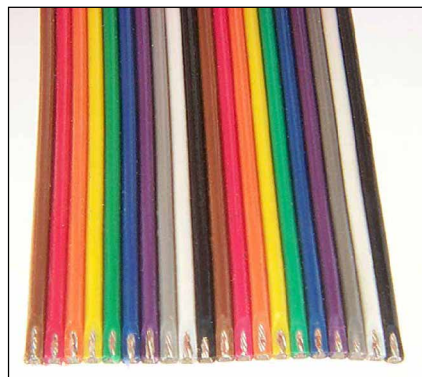
Figure 1—Standard ribbon cable prepared as described by KD5BIV. This is not the flat cable from a TH-79A.
