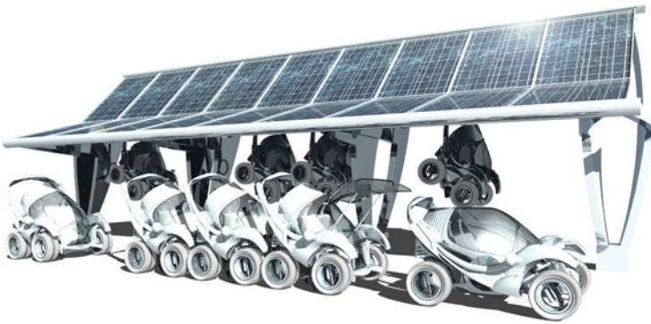
Fig. 12 S.O.F.T. Mobility: Stackable car. Urban stackable car with solar recharge port (Credits: Mitchell Joachim)
