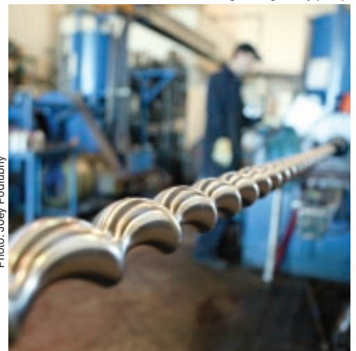
Progressing cavity pump.
