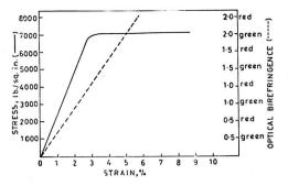
Fig. 1 — Stress-strain-optical birefringence characteristics of nylon copolymer at 72°F. and 14 per cent relative humidity [Gage length, 3 in.; cross-section, 0.25 in.  $\times$  0.0108 in.; value of elastic constant (E) = 320,000 lb./sq. in. Optical birefringence is expressed in terms of number of fringes observed as the strain is varied]
