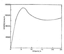
Fig. 3 -- Compression stress versus strain curve for polystyrene
