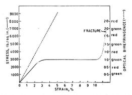
Fig. 2 — Stress-strain-optical birefringence characteristics of nylon copolymer at 72°F. and 46 per cent humidity [Gage length, 3 in.; cross-section, 0.25 in. $\times$ 0.0108 in.; value of elastic constant (E) = 130,000 lb./sq. in. Optical birefringence is expressed in terms of number of fringes observed as the strain is varied]
