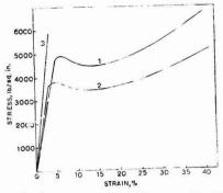
Fig. 4 — Tensile stress versus strain curves for cellulose nitrate (curve 1), cellulose acetate (curve 2) and polystyrenc (curve 3)
