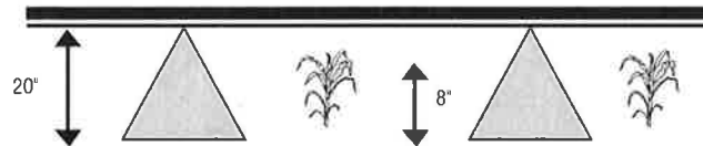
Diagram 1: Spray pattern of an even spray nozzle for inter-row applications.
