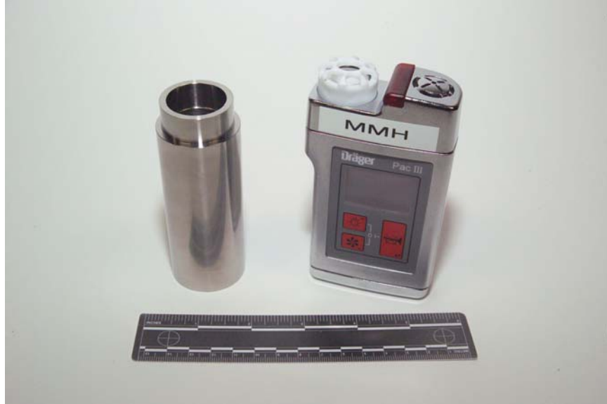
Figure 1 Headspace Analysis Container and Dräger PAC III Hydrazine Vapor Monitor
