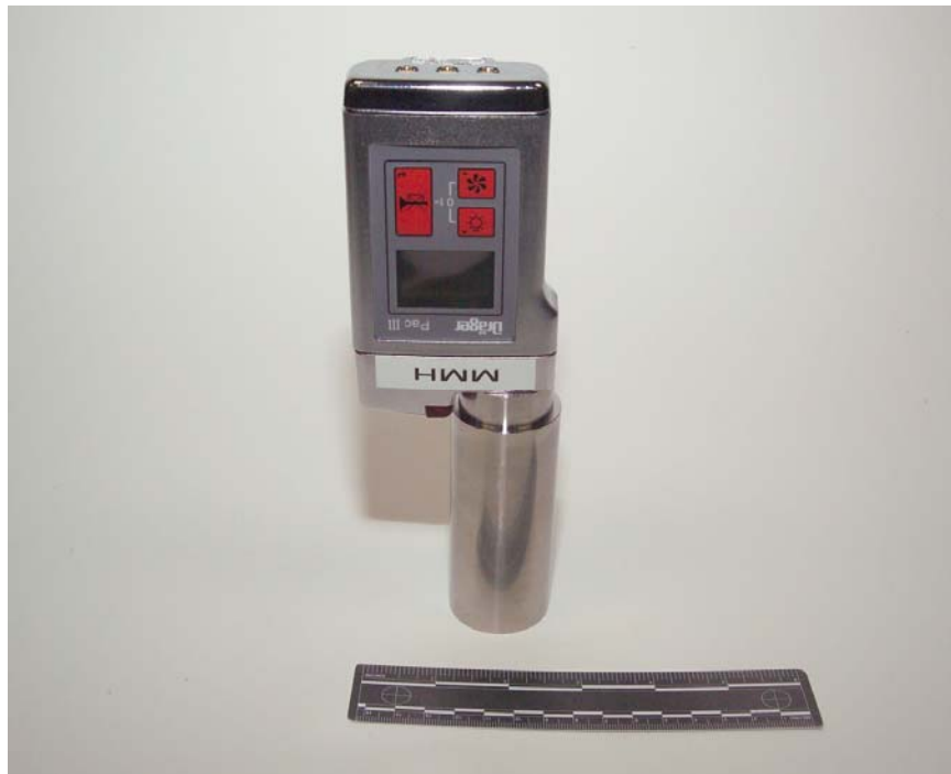
Figure 2 Headspace Analysis Container Fitted to Dräger PAC III Hydrazine Vapor Monitor
